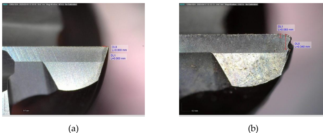
Figure 7. (a) Image of fresh cutting tool under parameter set 1 (1500 rpm, 0.75 mm, 225 mm/min) (b) Image of worn cutting tool under parameter set 1 (1500 rpm, 0.75 mm, 225 mm/min)
