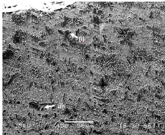
Figure 6. location near the arc source showing many reprecipitation of TiC structures with (i) of a flower type of TiC and (ii) globular.
