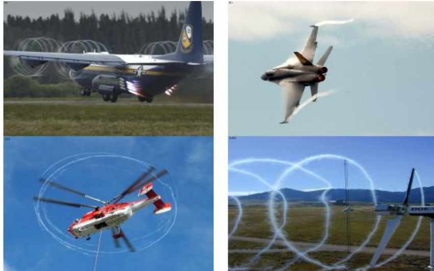
Figure 1: Helical vortices created from different devices such as from a: (a) propeller [4]; (b) wing [5]; (c) rotor [6]; and (d) blade [7].
