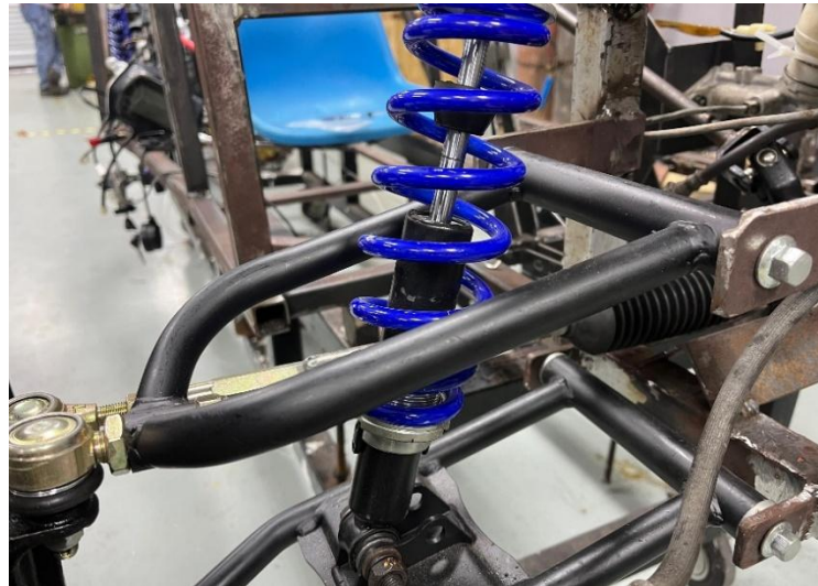
Figure 3: The upper arm when installed on the vehicle
