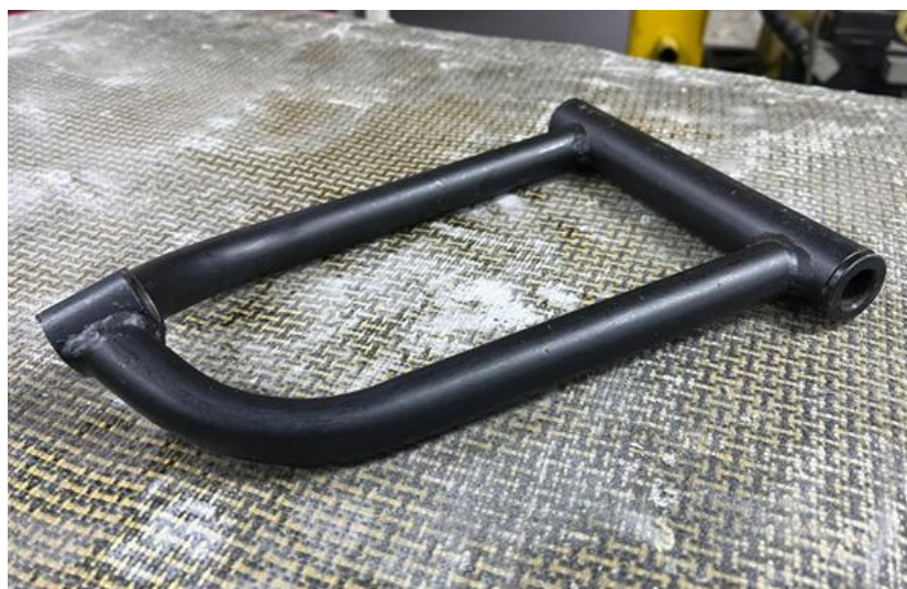
Figure 2: The actual design of the upper arm
