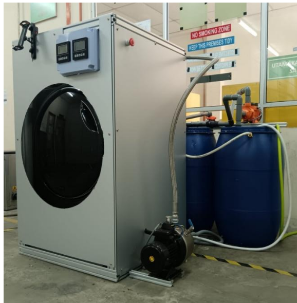
Figure 4: Final prototype of eco-friendly batik processing machine
