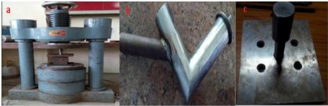
Figure 2: Experimental setup of powder metallurgy process (a) Compaction machine (b) Blender (c) die used in making the samples
