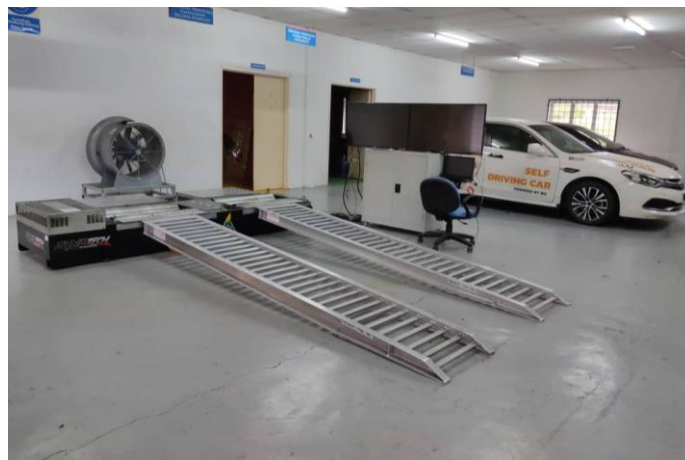
Figure 3: Dyno-Dynamics Chassis Dynamometer setup
