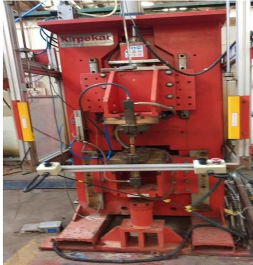
Figure 1. Kirperker RSW welding machine
