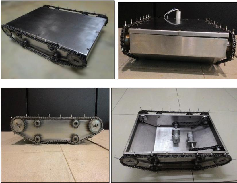
Figure 5. The prototype of ROC inside view.
