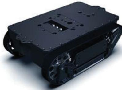
Figure 2. Hull Crawler by Qinetiq North America. (Jansen, G.,2013)
