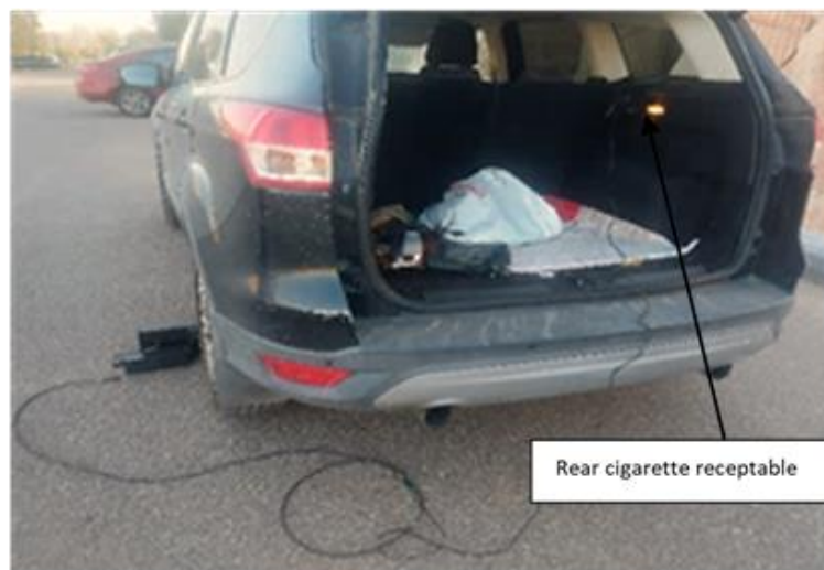
Figure 8: Modified jack connected to the vehicle battery using cigarette lighter receptable.
