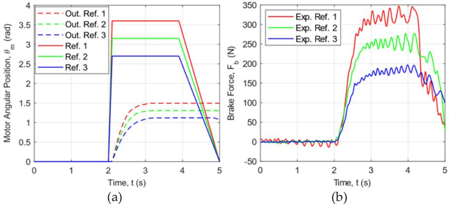
Figure 3: EWB prototype responses (a) Control target and actual (b) Brake force
