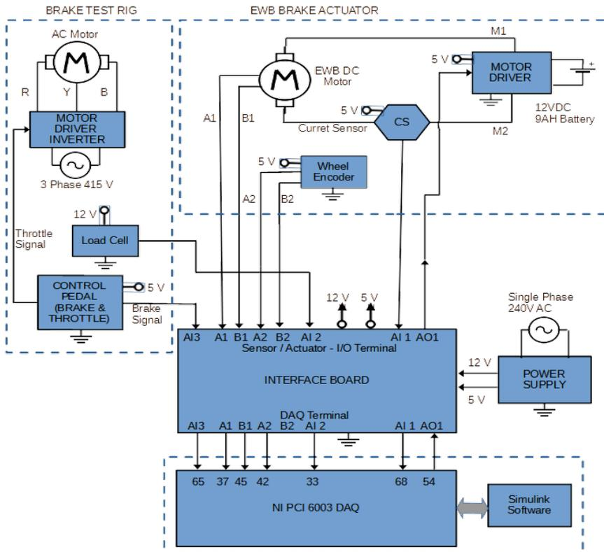
Figure 2: The EWB experimental wiring connection
