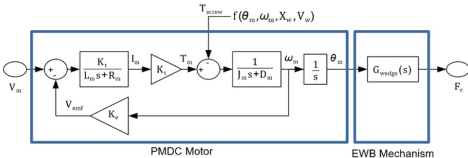
Figure 1: Overall EWB frequency-based block diagram
