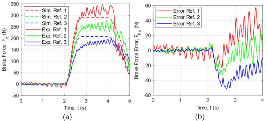
Figure 6: Brake force - simulation vs experimental (a) Response (b) Response error
