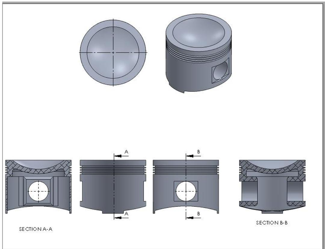
Figure 6: The sectional view of the modelled conventional piston
