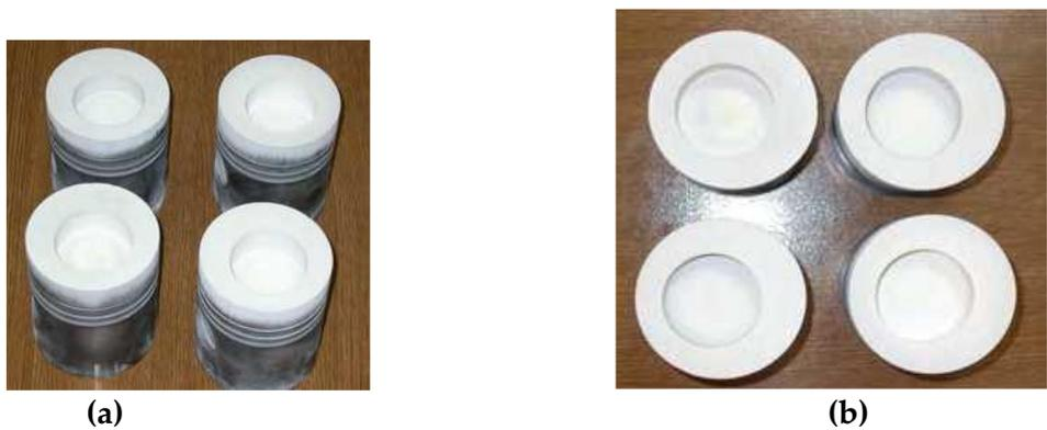
Figure 3: Ceramic coated piston tops
