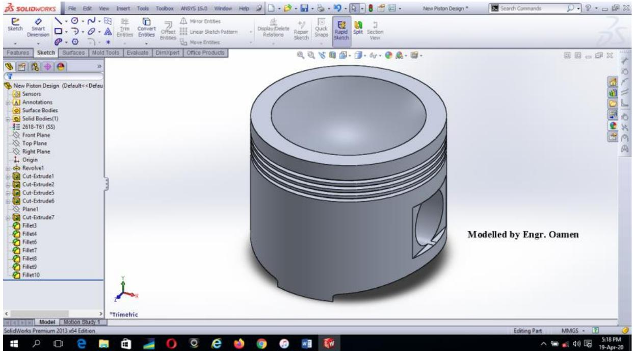
Figure 5: The isometric view of the 3D modelled conventional piston
