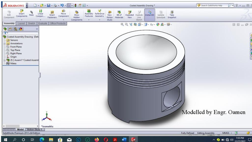
Figure 9: The assembly view of the reconditioned piston with bond and topcoat layers
