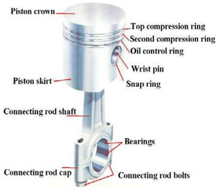
Figure 1: The different parts or elements of the piston
