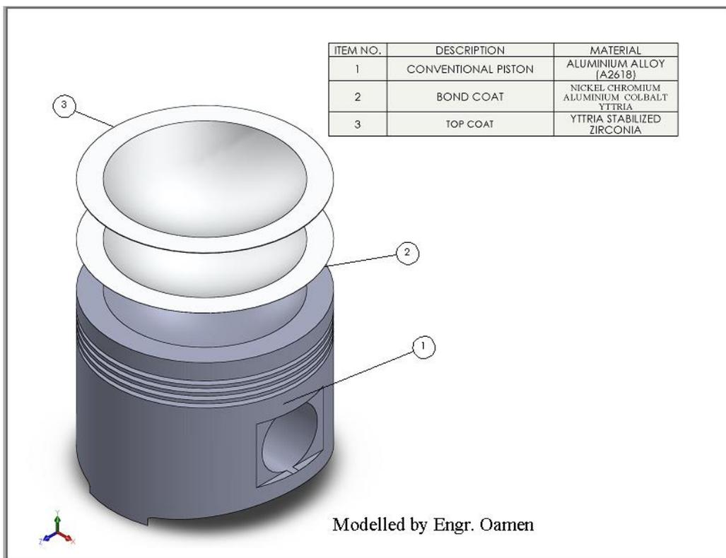
Figure 10: The exploded view of the reconditioned piston with bond and topcoat layers
