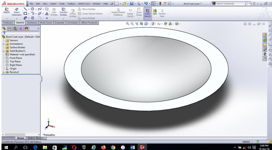
Figure 7: The modelled isometric view of the bond-coat layer of 0.15 thickness
