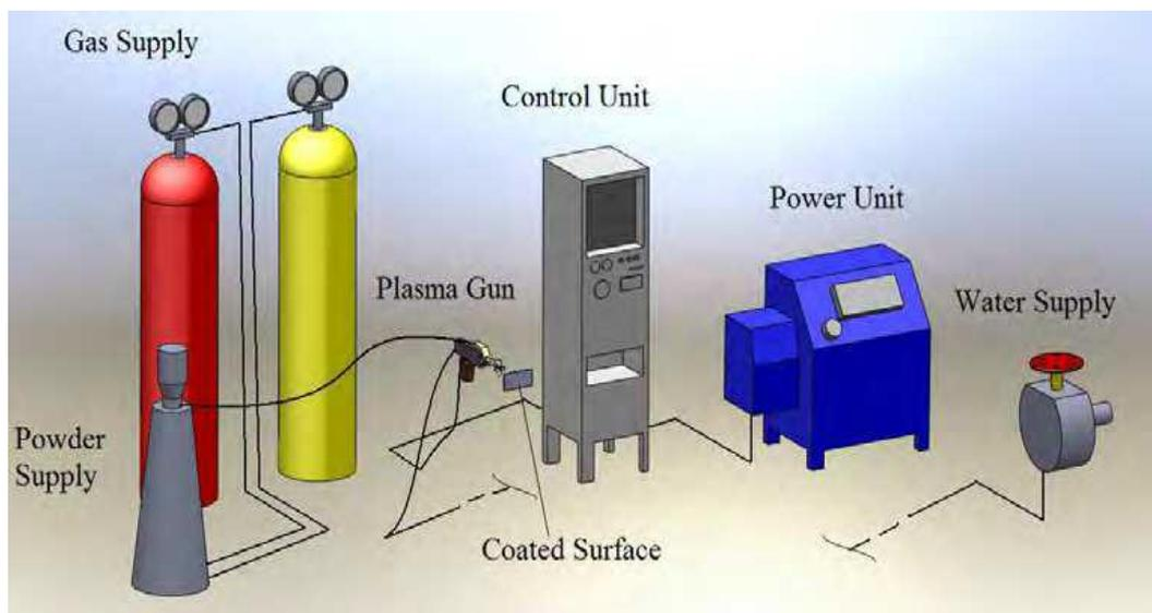
Figure 2: Plasma spray-coating system
