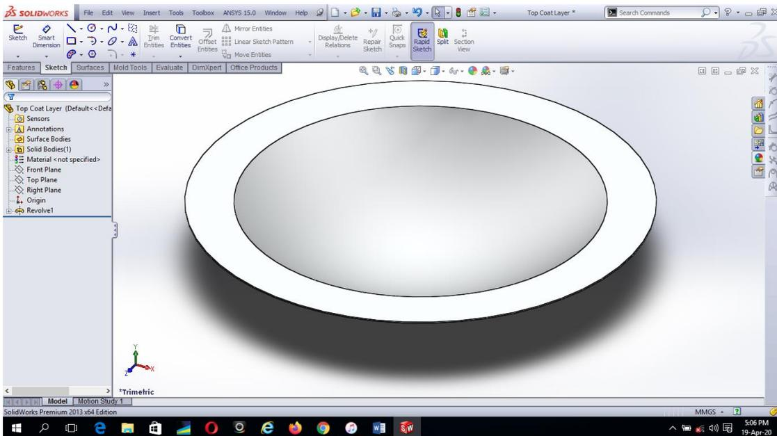
Figure 8: The modelled isometric view of the topcoat layer of 0.35 thickness
