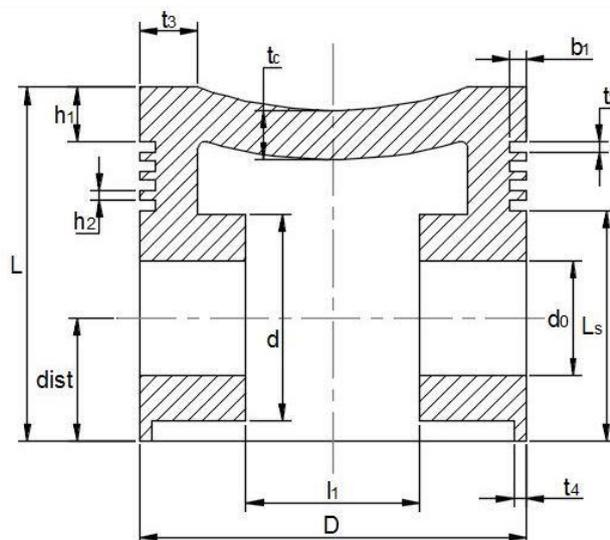
Figure 4: Cross-section of the model conventional piston
