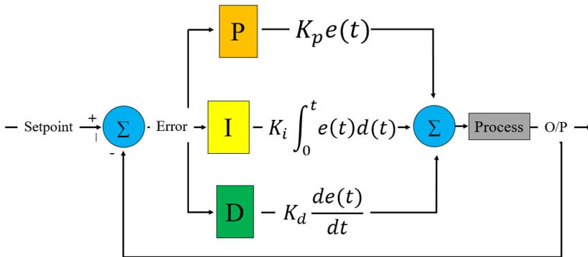
Figure 2: The designed PID controller in Simulink
