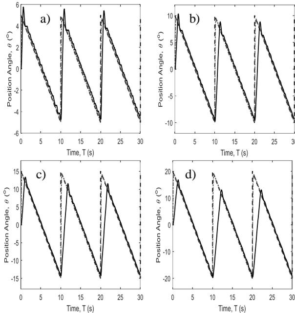
Figure 8: Responses of position tracking control in saw tooth function for a) 5°, b) 10°, c) 15° and d) 20°
