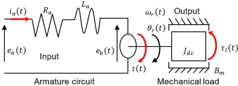
Figure 1: Schematic diagram of DC motor
