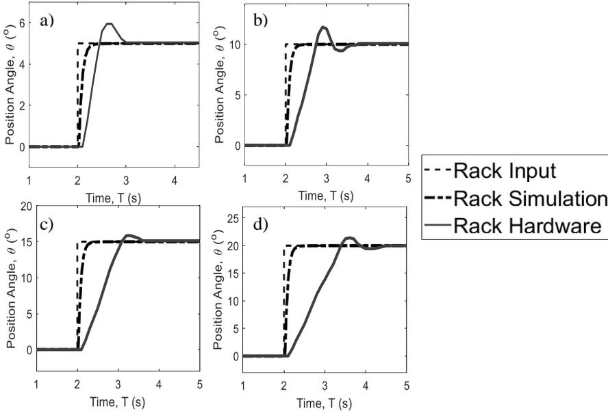
Figure 6: Responses of position tracking control for step function for; a) 5°, b) 10°, c) 15° and d) 20°
