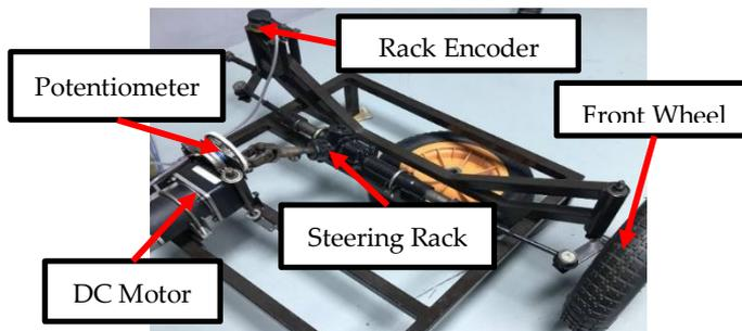
Figure 4: Front Wheel System Test Rig
