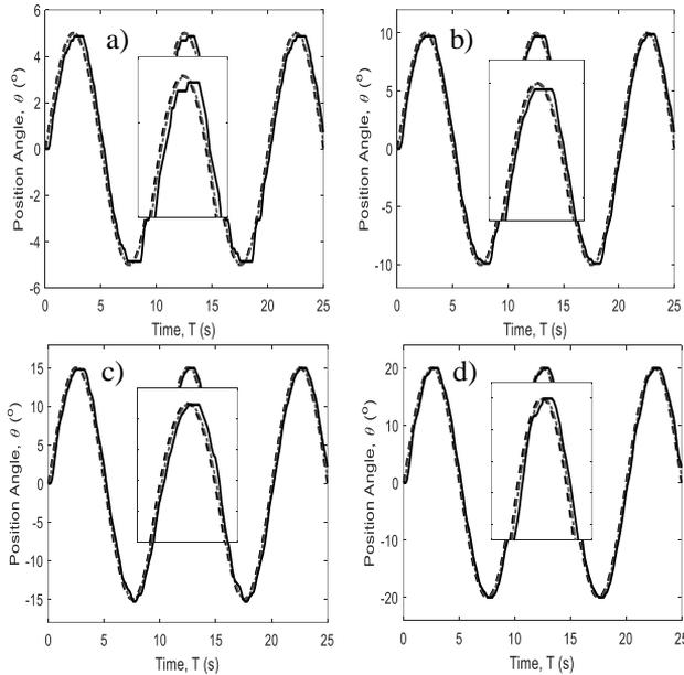
Figure 7: Responses of position tracking control in sine function for; a) 5°, b) 10°, c) 15° and d) 20°
