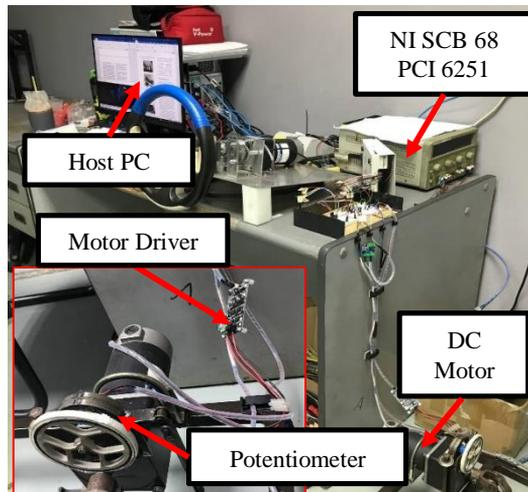
Figure 5: HiLS setup for position tracking of DC motor
