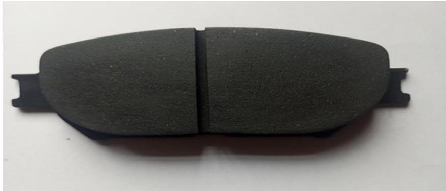
Figure 10: Finished CAW-based Brake Pad with 90  $\mu\text{m}$  particle size
