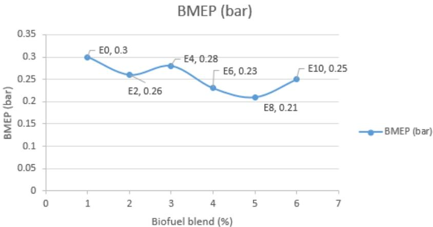
Figure 7: The BMEP (bar) of an engine with different ethanol blend (%)
