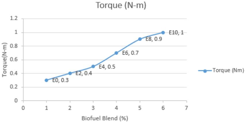
Figure 4: The engine torque (N/m) with ethanol blend (%)
