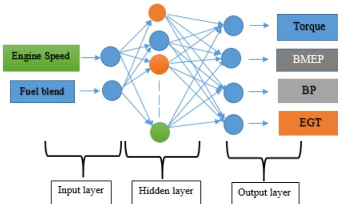
Figure 3: Artificial neural network for predicting engine performance characteristics of biofuel
