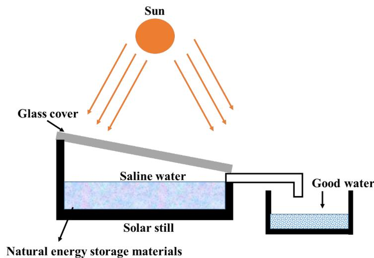
Figure 5. Principle of solar still
