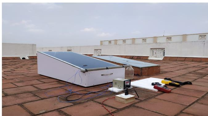
Figure 1. Constructional view of solar still
