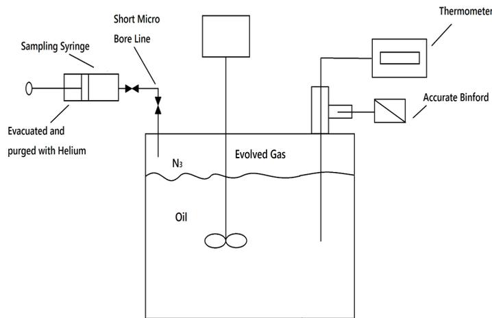
Figure 3. Equipment arrangement for experimental analysis (Husain et al., 2003)
