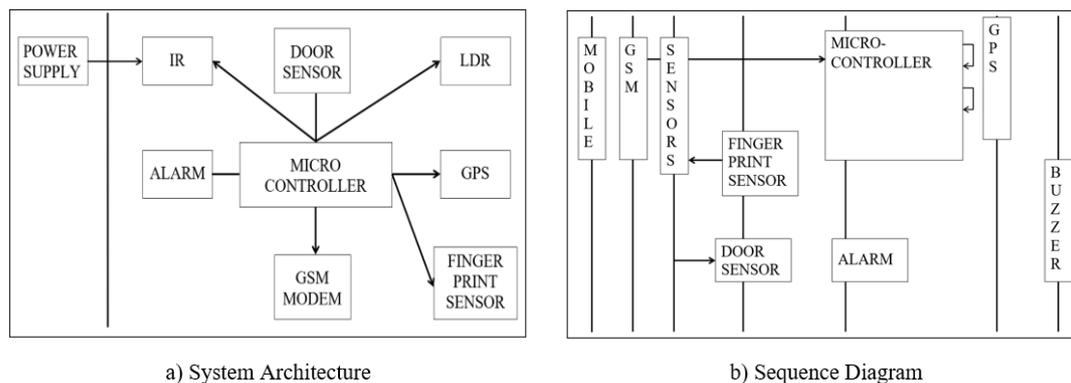
Figure 5. System architecture and sequence diagram of the proposed system (Dinesh, 2017)
