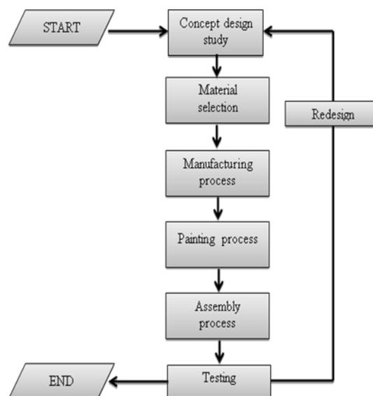
Figure 2: Design process of low-cost manually operated bending machine
