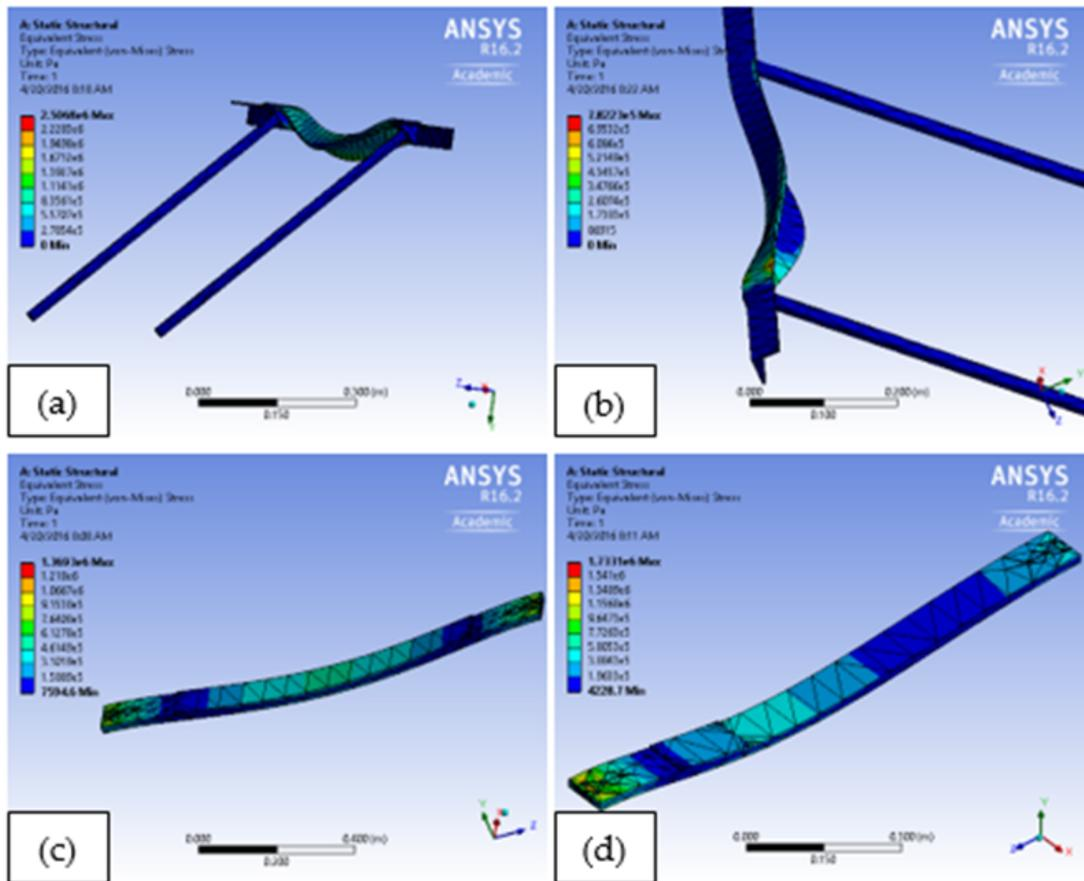
Figure 6: Stress analysis for (a) bender plate for a large sample, (b) bender plate for a small sample, (c) bending base for a large sample, and (d) bending base for small sample
