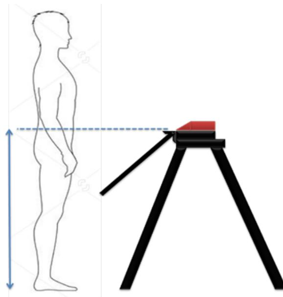
Figure 3: Proposed height of bending machine according to Anthropometric data
