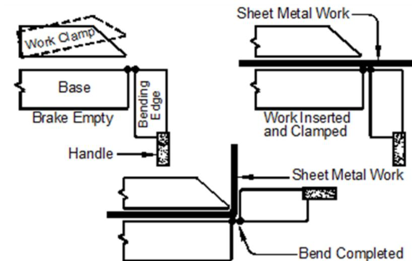
Figure 1: Basic principle of bending machine
