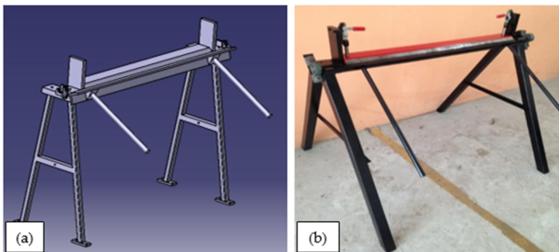
Figure 4: Image of designed bending machine (a) drawing and (b) fabricated
