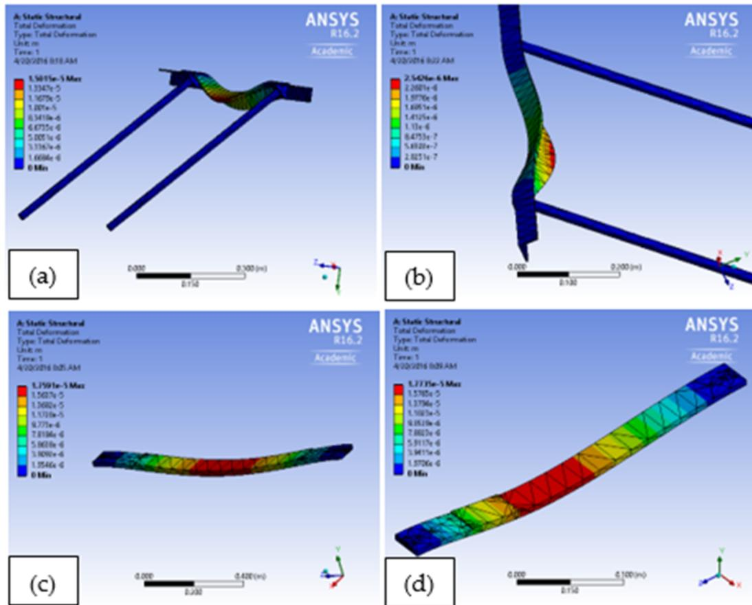
Figure 7: Deflection analysis for (a) bender plate for a large sample, (b) bender plate for a small sample, (c) bending base for a large sample, and (d) bending base for small sample
