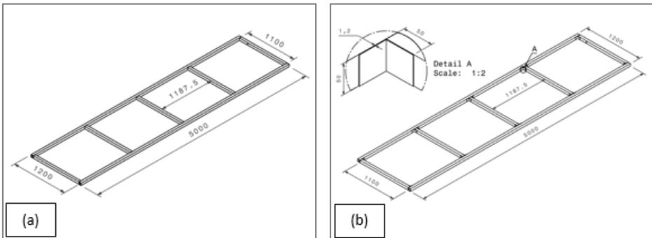
Figure 1: Detail dimension for (a) thin-walled chassis and (b) thin-walled chassis with gusset plate
