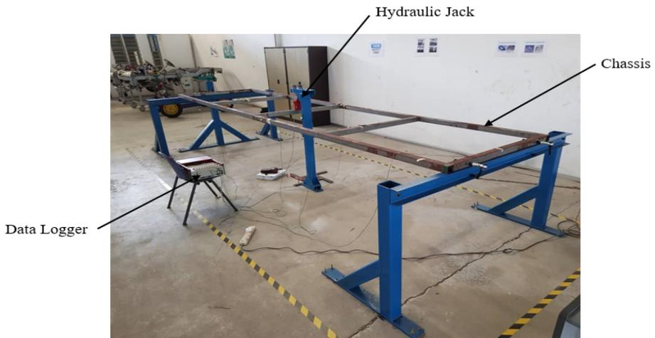
Figure 2: Experimental setup for the loading condition of the chassis
