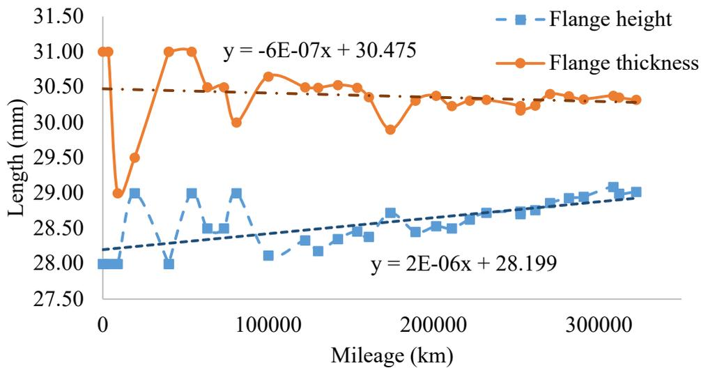
Figure 22: Railway wheel profile data for wheel 9L
