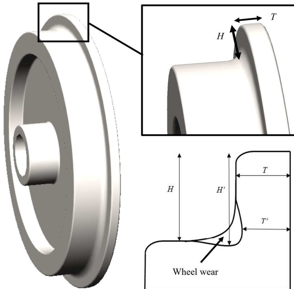
Figure 3: Wheel flange height and flange thickness
