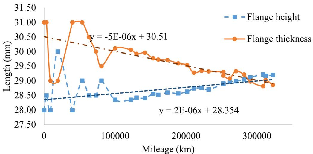
Figure 21: Railway wheel profile data for wheel 8L
