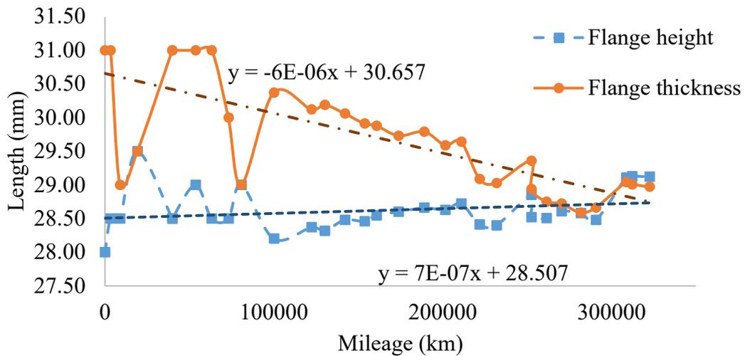
Figure 11: Railway wheel profile data for wheel 8R
