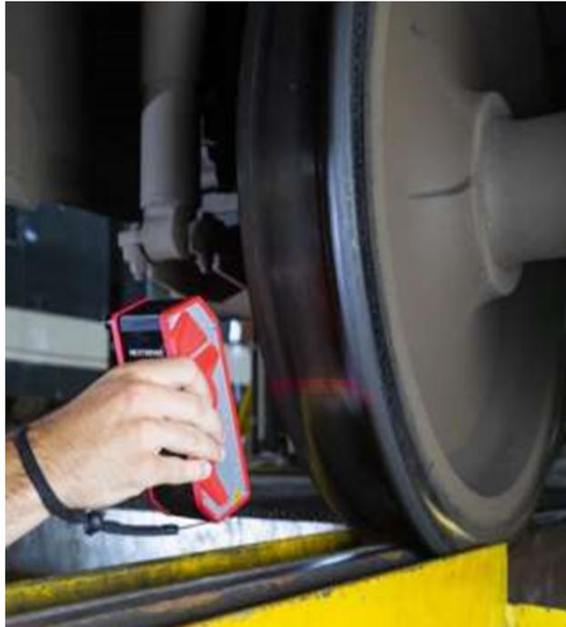
Figure 2: Calipri wheel measurement device
