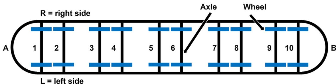
Figure 1: Orientation of the wheel and axle on the train [12-14]
