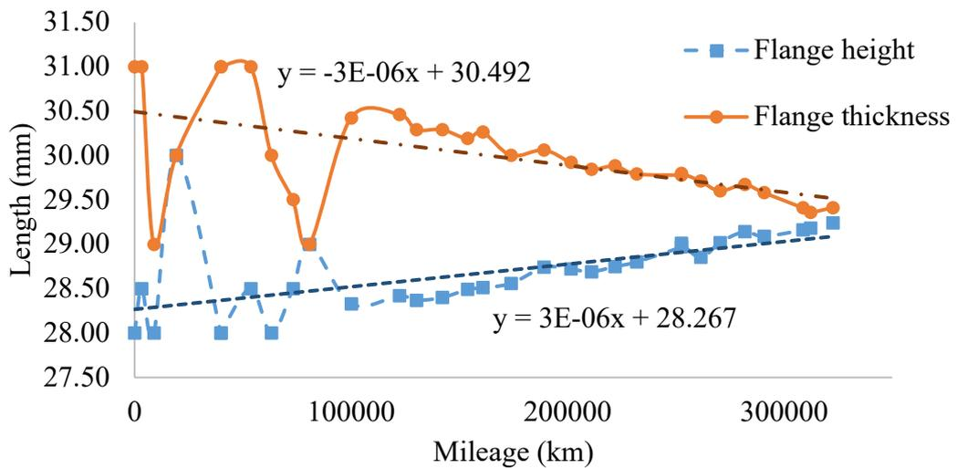
Figure 17: Railway wheel profile data for wheel 4L
