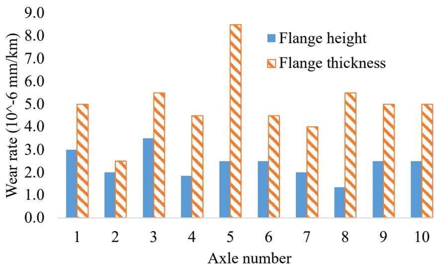
Figure 26: Average wear rate on the different axle
