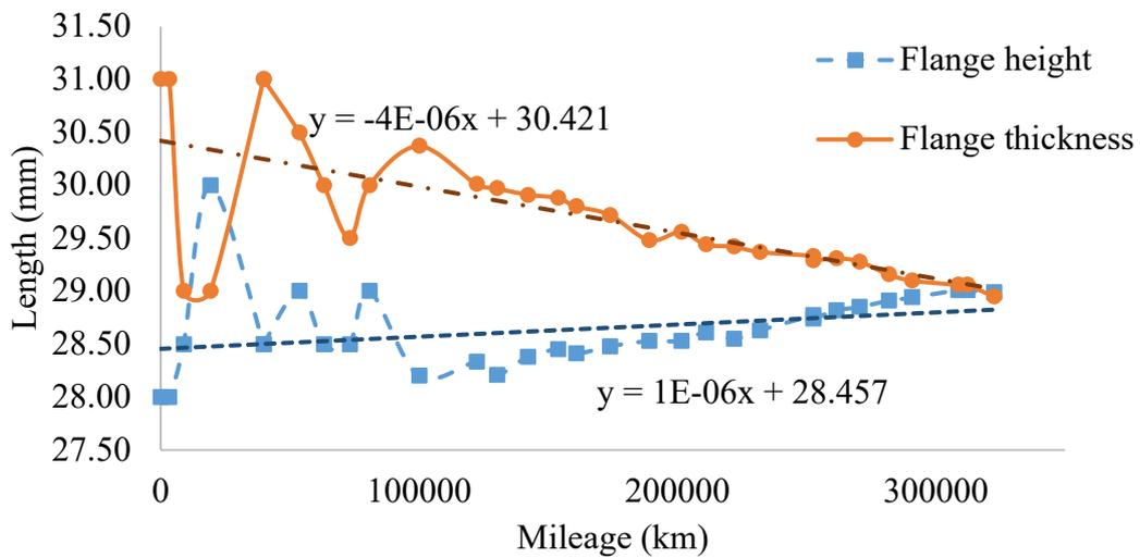
Figure 20: Railway wheel profile data for wheel 7L
