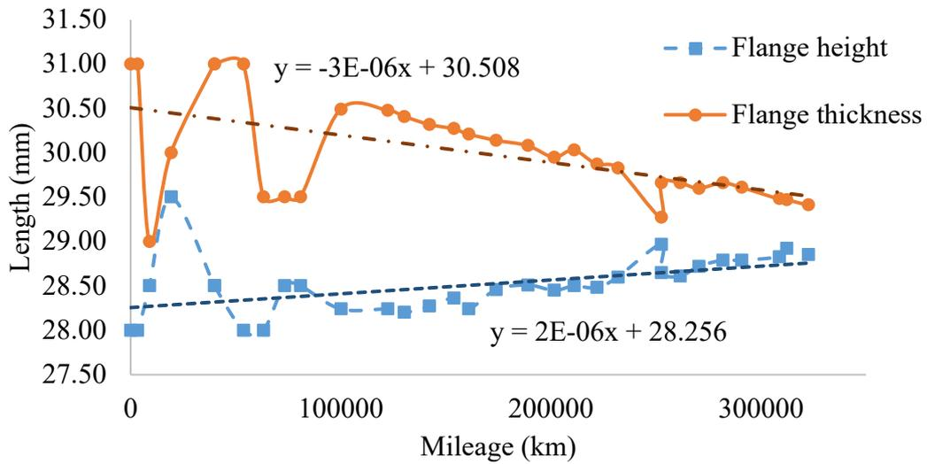
Figure 5: Railway wheel profile data for wheel 2R
