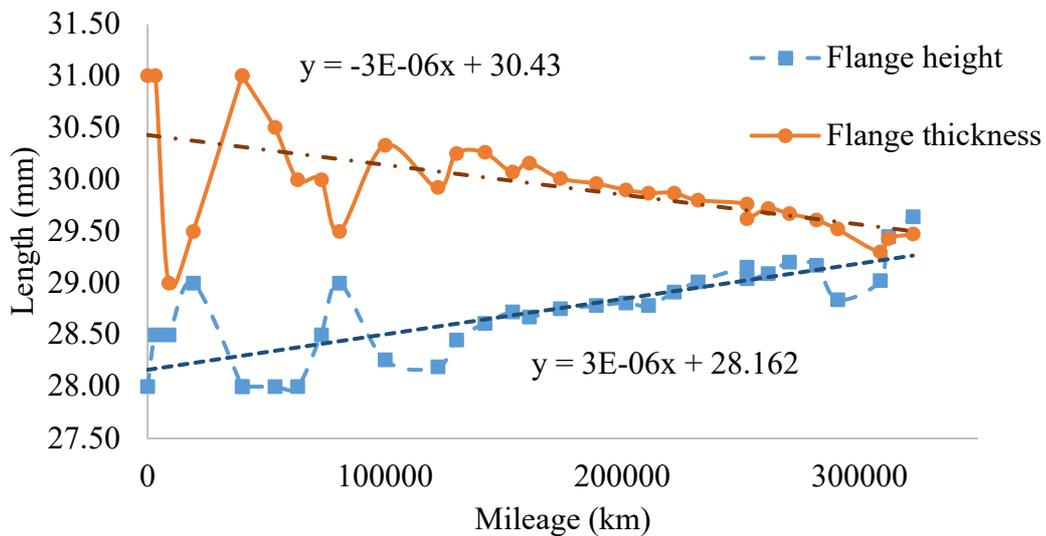
Figure 23: Railway wheel profile data for wheel 10L
