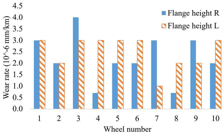
Figure 28: Wear rate of flange height
