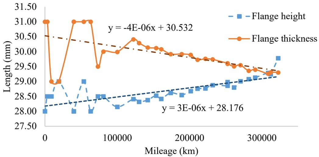
Figure 10: Railway wheel profile data for wheel 7R
