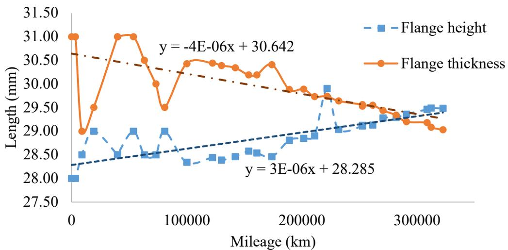
Figure 12: Railway wheel profile data for wheel 9R
