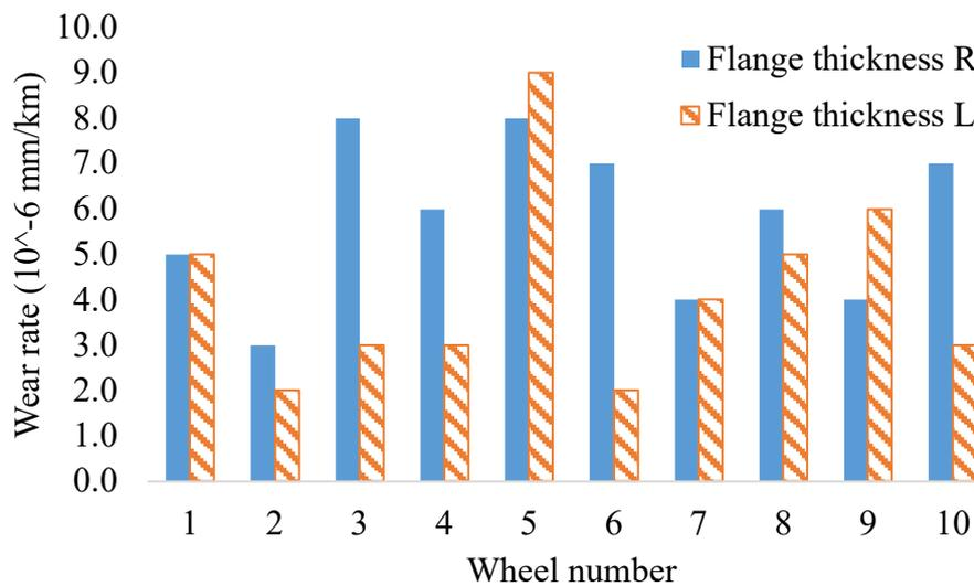
Figure 29: Wear rate of the flange thickness
