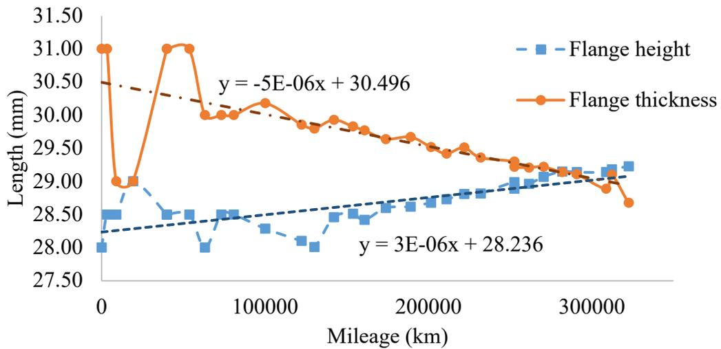
Figure 14: Railway wheel profile data for wheel 11L
