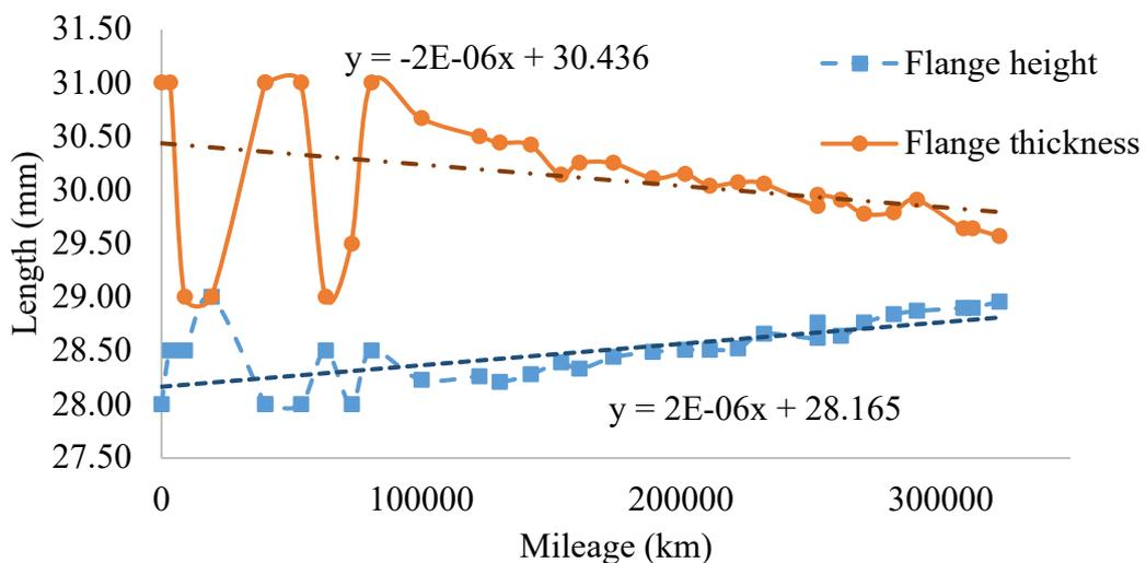
Figure 15: Railway wheel profile data for wheel 2L
