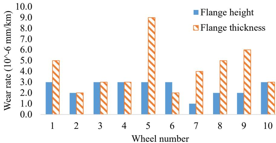
Figure 25: Wear rate of left flange height and thickness
