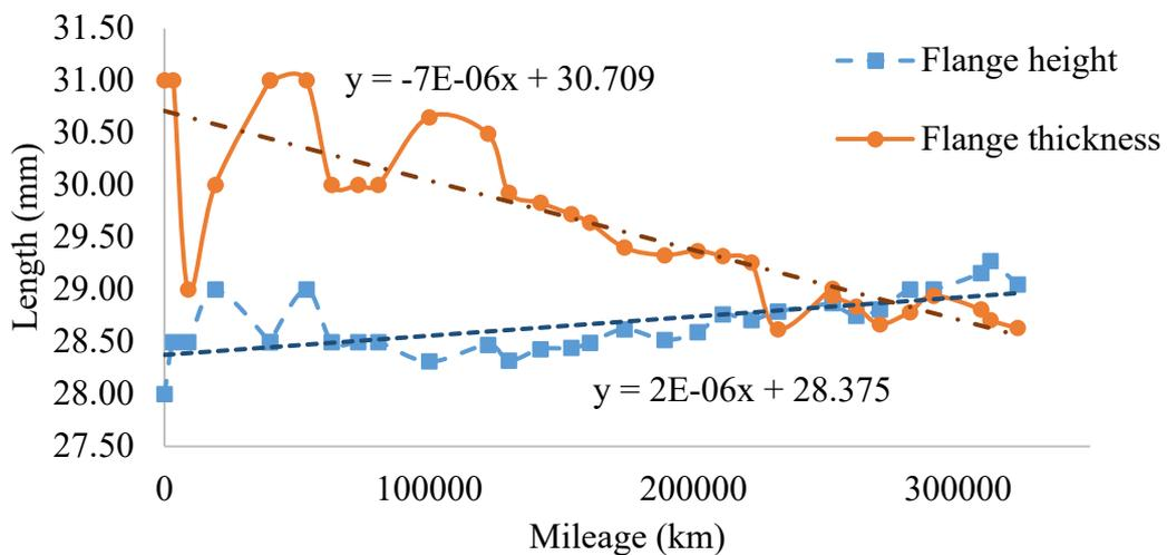
Figure 9: Railway wheel profile data for wheel 6R
