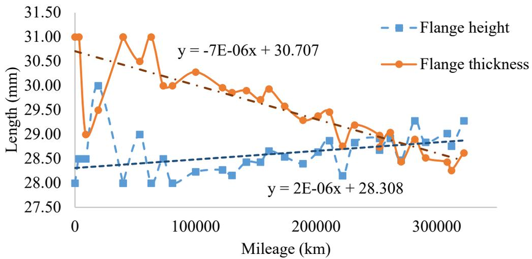
Figure 13: Railway wheel profile data for wheel 10R
