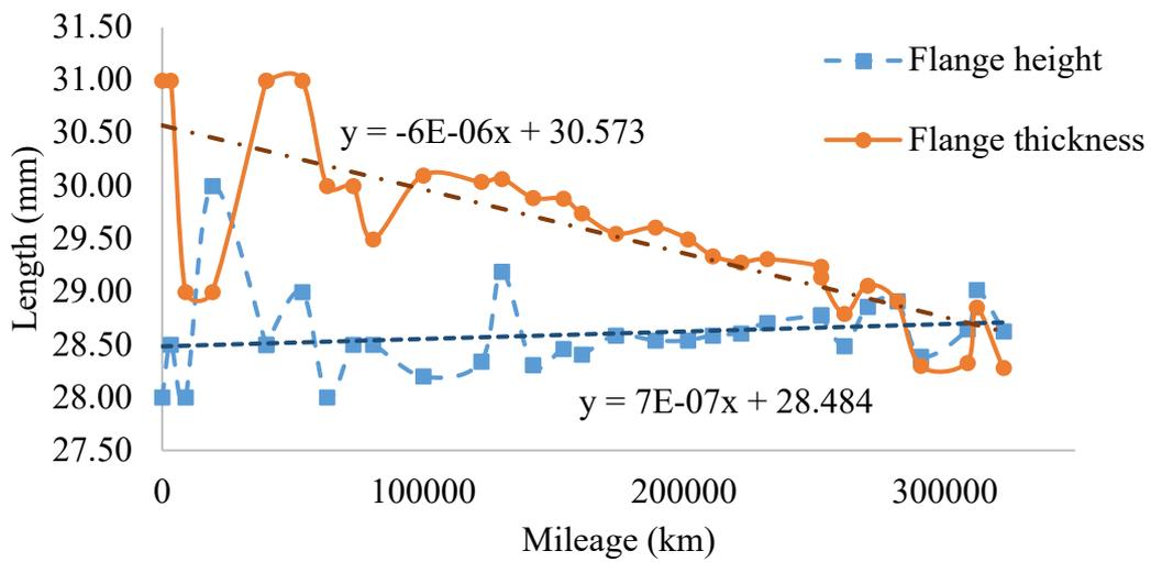
Figure 7: Railway wheel profile data for wheel 4R
