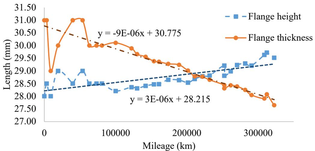
Figure 18: Railway wheel profile data for wheel 5L
