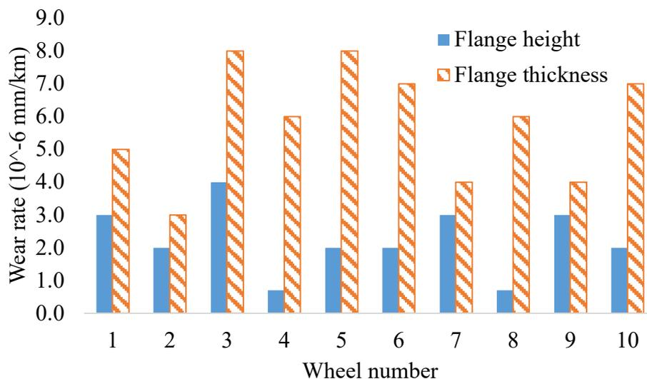
Figure 24: Wear rate of right flange height and thickness
