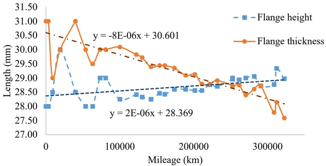
Figure 8: Railway wheel profile data for wheel 5R
