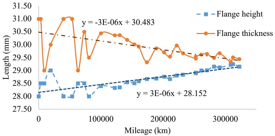
Figure 16: Railway wheel profile data for wheel 3L
