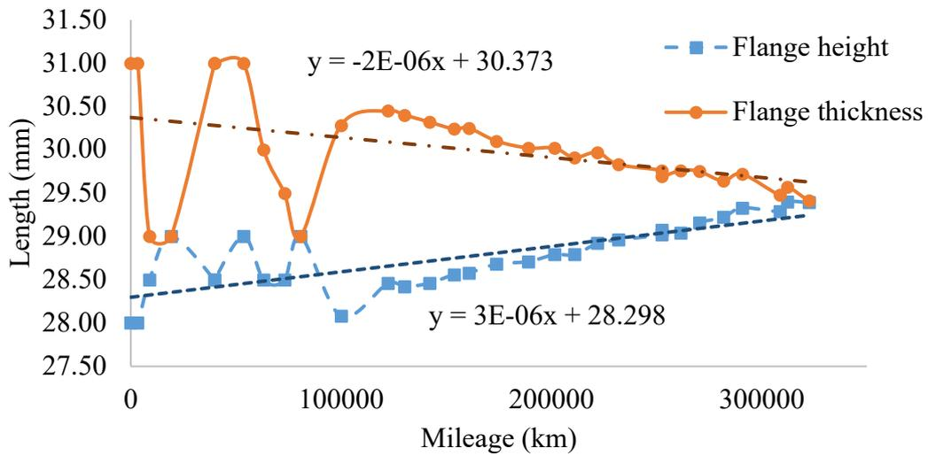
Figure 19: Railway wheel profile data for wheel 6L
