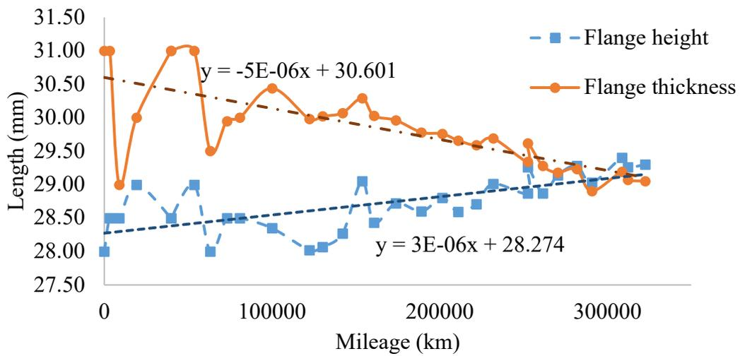
Figure 4: Railway wheel profile data for wheel 1R
