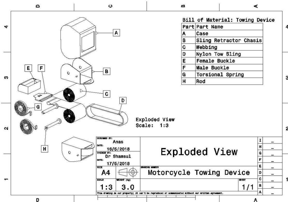
Figure 5. Exploded view of the device
