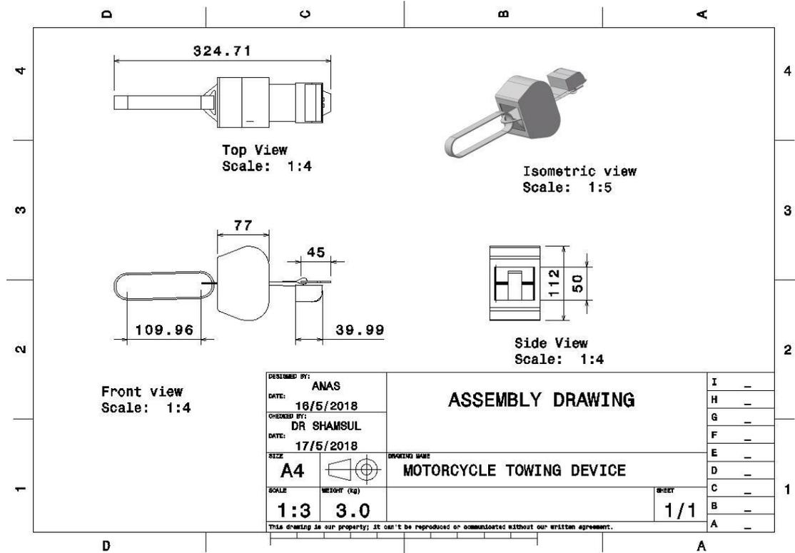
Figure 4. Assembly drawing for motorcycle towing device
