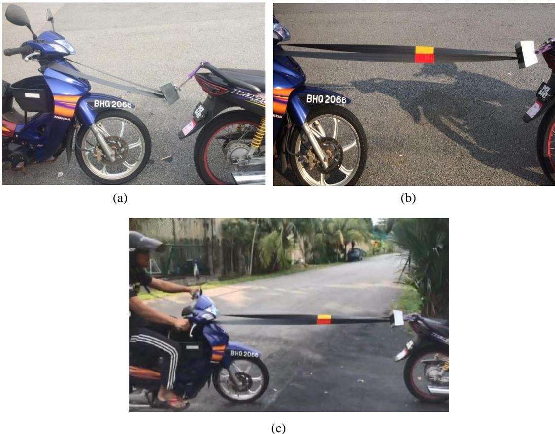
Figure 7. Application of the device on both vehicles for road test.
