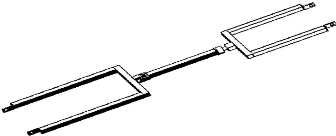
Figure 3. Towing device between two motorcycles (Hasif, 2015)
