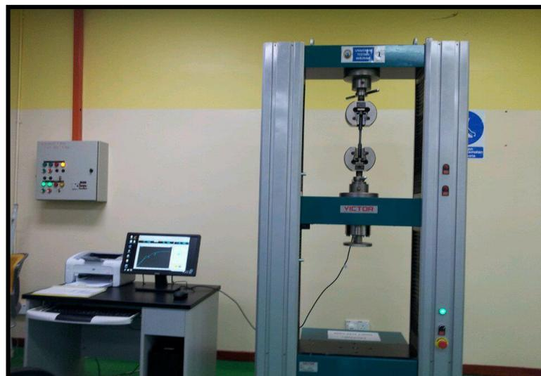
Figure 7. Tensile test machine (VEW 2302)
