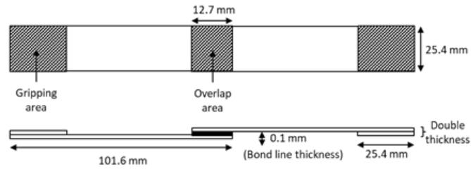
Figure 2. Sample assembly for single-lap bonded joint test
