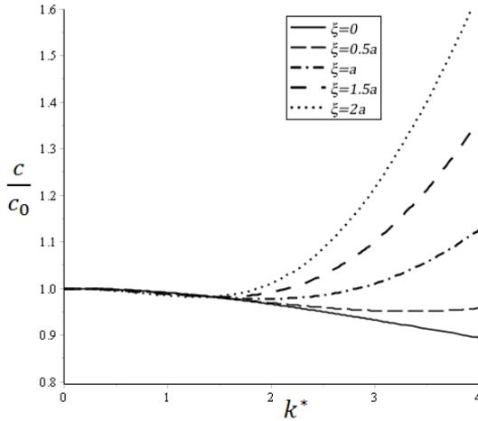
Figure 2. Effect of material parameter on velocity of stress wave propagation with  $\beta = 1$  and  $\nu=0.25$ .
