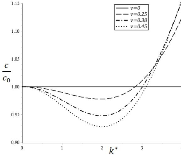
Figure 4. Poisson's effect on velocity of stress wave propagation with  $\beta = \mathbf{1}$  and  $\xi = \alpha$ .
