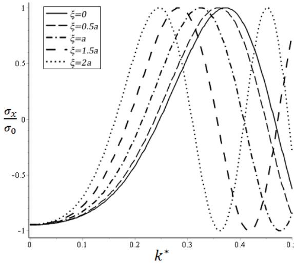
Figure 5. Behavior of non-dimensional axial stress wave versus non-dimensional wave number with different material length scale parameter under  $\beta = \mathbf{1}$ ,  $\nu=0.25$ ,  $x=10a$  and  $t=0.1s$ .
