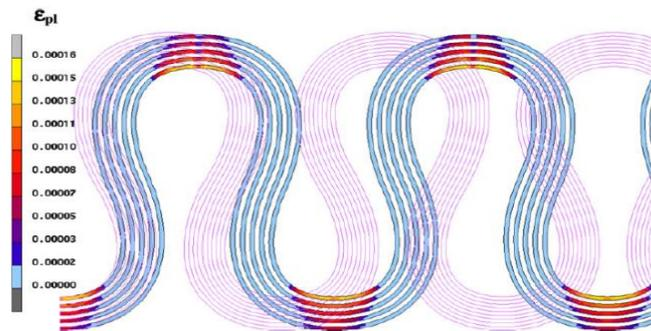
Figure 6. Plastic strain distribution in a multi-track horseshoe conductor design (Gonzalez et al., 2008)
