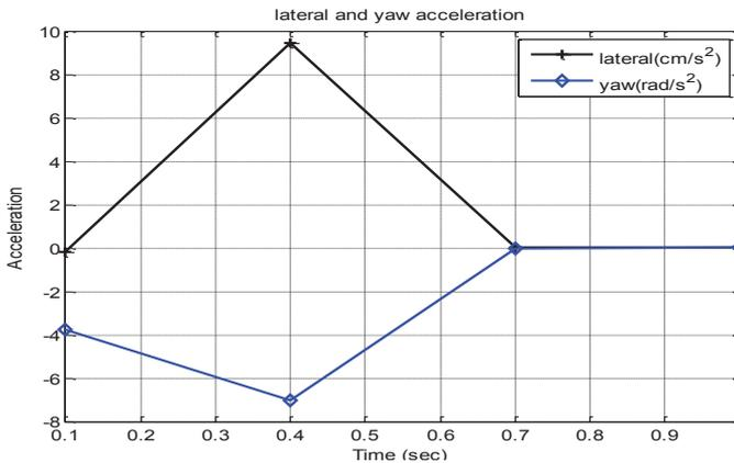
Figure 6. Acceleration of lateral and yaw of rail wheelset
