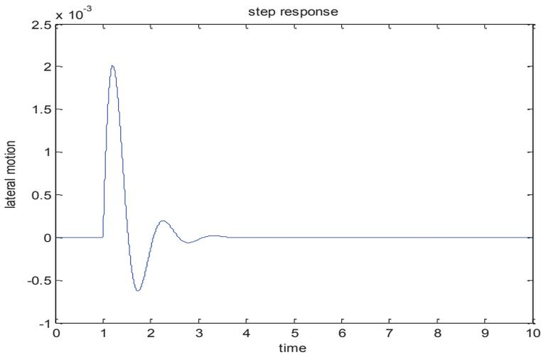
Figure 7. Step response of lateral motion of rail vehicle wheelset
