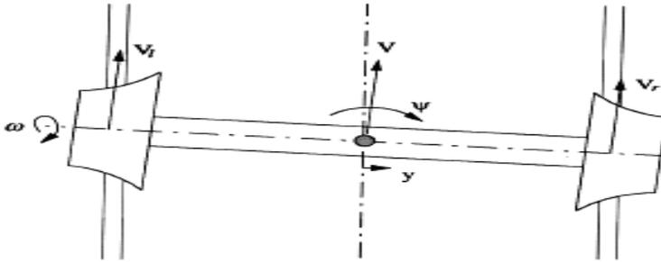
Figure 1. Rail wheelset geometry showing lateral and yaw motion
