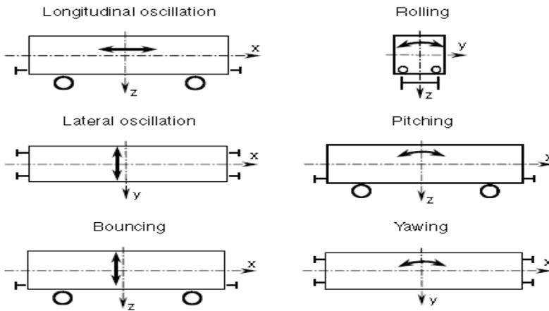
Figure 2. Possible Types of motions created by rail vehicle during running
