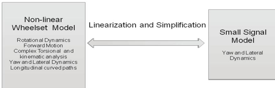
Figure 3 . Schematic Diagram from non-linear to linear modeling
