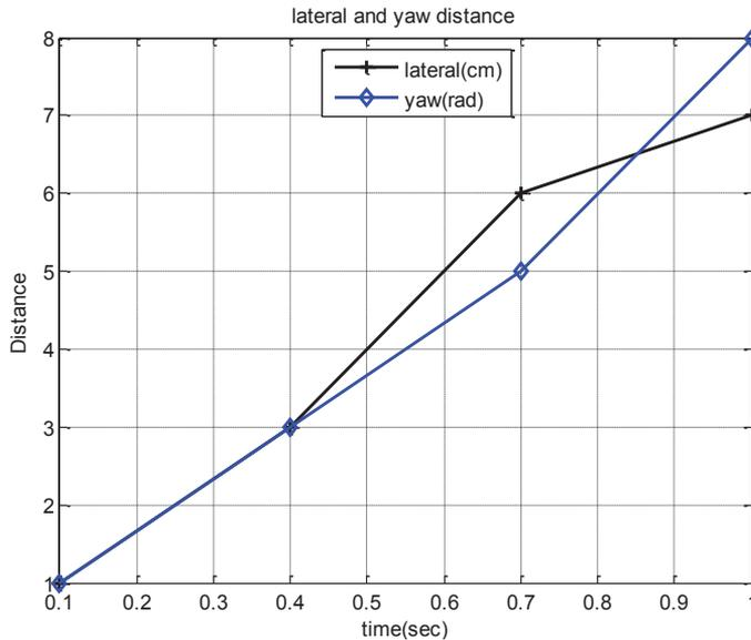
Figure 4 Relation of lateral and yaw displacement of rail wheelset
