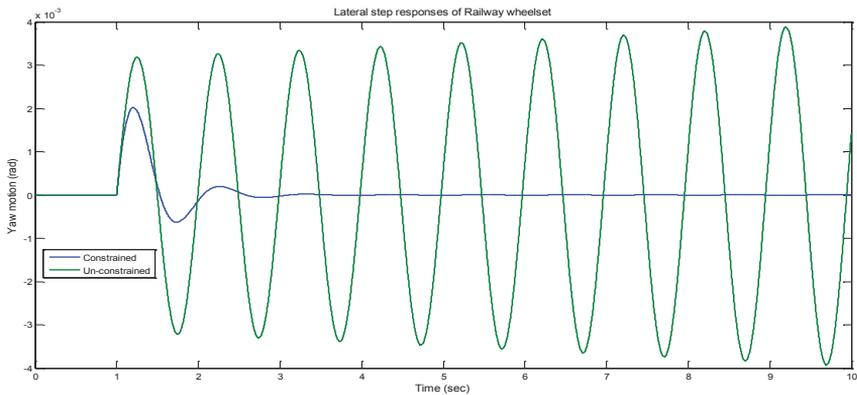
Figure 8. Constrained and unconstrained yaw motion of rail locomotive
