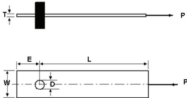
Figure 2. Geometry of the Specimen
