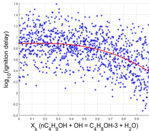
Figure 11. Component function for TRF/*n*-butanol mixture at  $T = 858$  K with respect to  $n\text{-C}_4\text{H}_9\text{OH} + \text{OH} = \text{C}_4\text{H}_8\text{OH-3} + \text{H}_2\text{O}$ .
