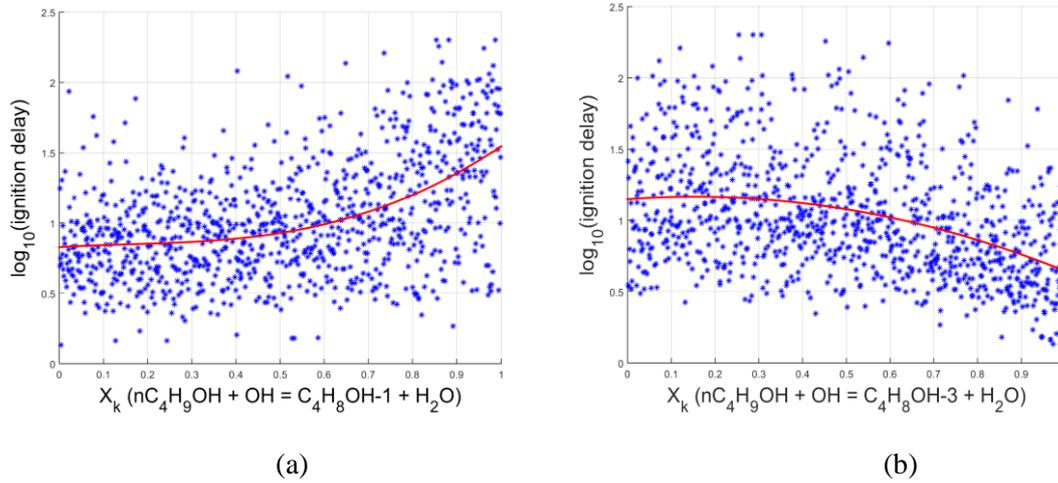
Figure 10. Component function for TRF/*n*-butanol mixture at  $T = 761$  K with respect to (a)  $n\text{-C}_4\text{H}_9\text{OH} + \text{OH} = \text{C}_4\text{H}_8\text{OH-1} + \text{H}_2\text{O}$  (b)  $n\text{-C}_4\text{H}_9\text{OH} + \text{OH} = \text{C}_4\text{H}_8\text{OH-3} + \text{H}_2\text{O}$ .
