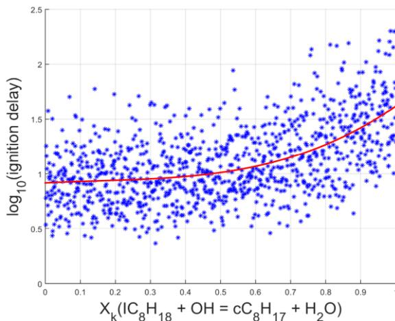
Figure 4. HDMR component functions (solid line) of simulated TRF ignition delays shown on-top of the scatter.  $P = 20$  bar,  $\phi = 1$ ,  $T = 761$  K. Sensitivity with respect to  $\text{IC}_8\text{H}_{18} + \text{OH} = \text{cC}_8\text{H}_{17} + \text{H}_2\text{O}$ .
