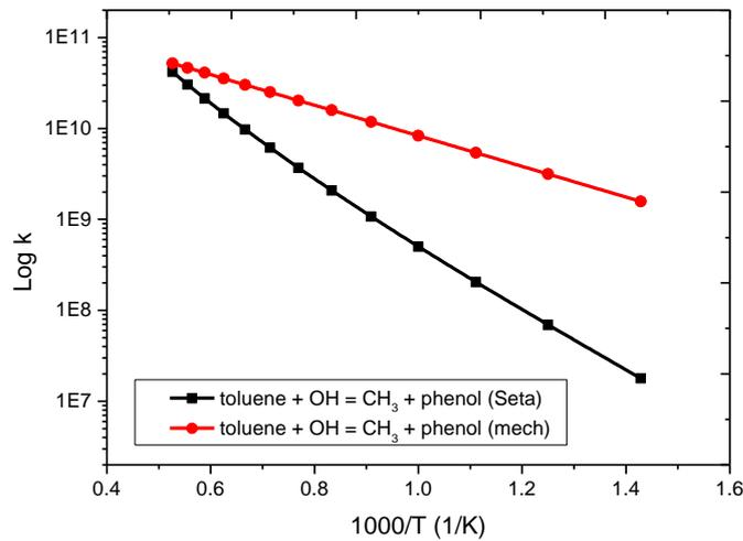
Figure 14. Comparison of the reversed rates of the phenol route (toluene + OH = phenol + CH<sub>3</sub>) captured in the LLNL mechanism with those estimated from the data of Seta (Seta et al., 2006).
