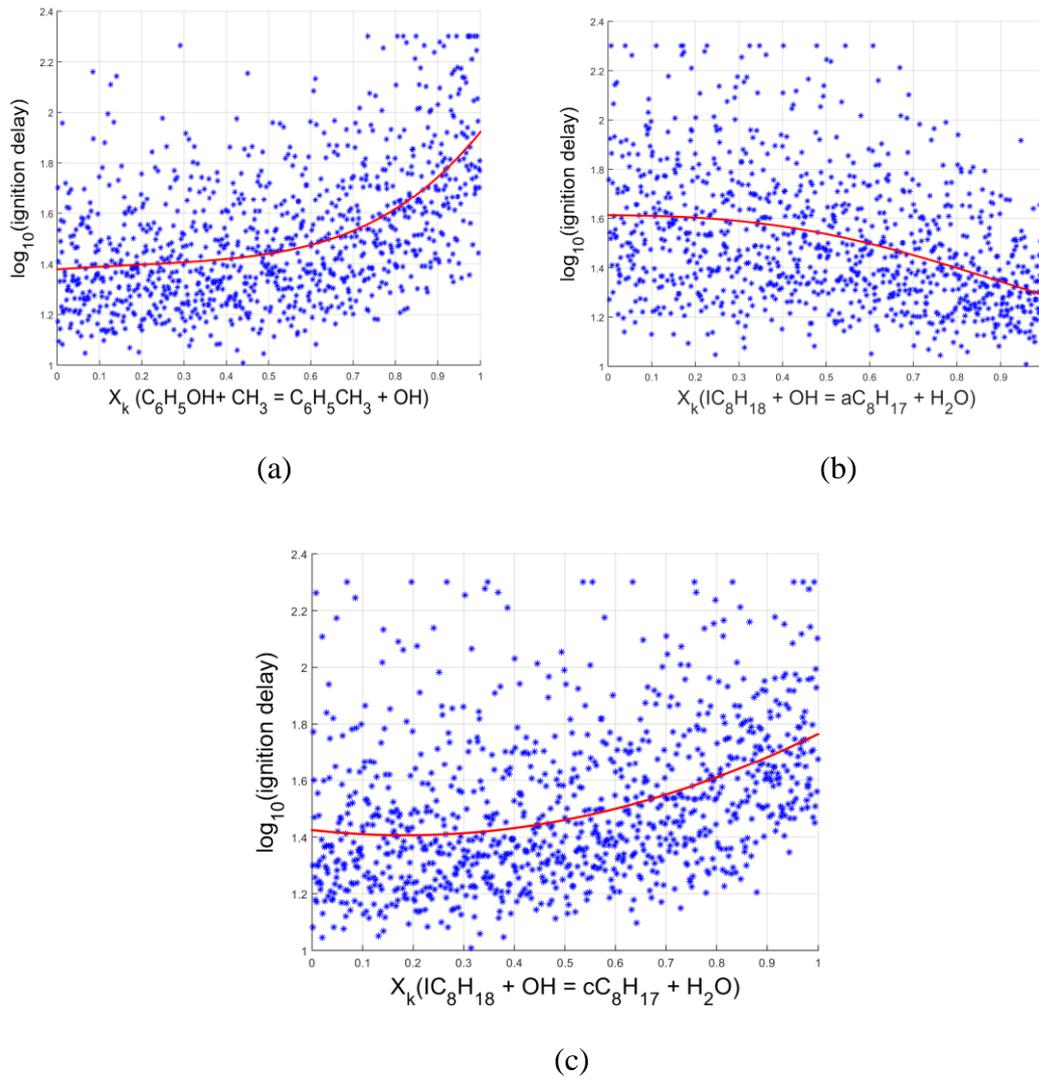
Figure 3. HDMR component functions (solid line) of simulated TRF ignition delays shown on-top of the scatter.  $P = 20$  bar,  $\phi = 1$ ,  $T = 679$  K. Sensitivity with respect to (a)  $\text{CH}_3 + \text{C}_6\text{H}_5\text{OH} = \text{C}_6\text{H}_5\text{CH}_3 + \text{OH}$  (b)  $\text{IC}_8\text{H}_{18} + \text{OH} = \text{aC}_8\text{H}_{17} + \text{H}_2\text{O}$  (c)  $\text{IC}_8\text{H}_{18} + \text{OH} = \text{cC}_8\text{H}_{17} + \text{H}_2\text{O}$ .
