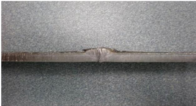
**FIGURE 2.4** Weld pool 0.8mm, 60V
