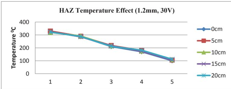
FIGURE 2.7 Temperature variations for 1.2mm, 30V
