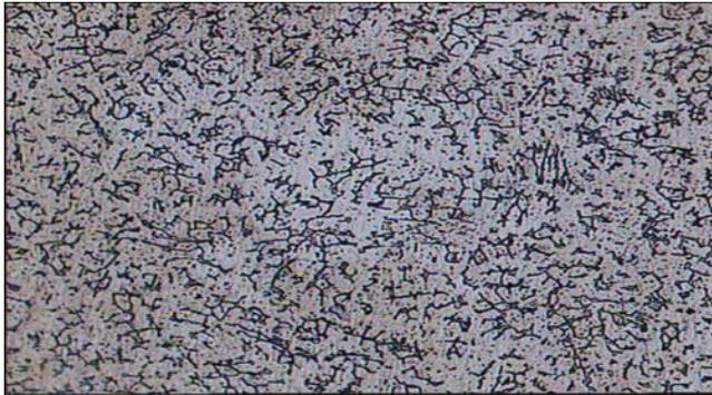
**FIGURE 2.15** Weldment area (100X magnification : 1.0mm, 30v)
