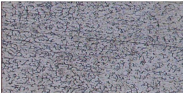
**FIGURE 2.13** Weldment area (100X magnification : 0.8mm, 30v)
