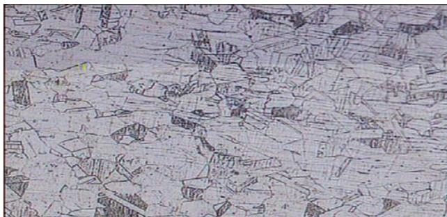
**FIGURE 2.14** HAZ (100X magnification: 1.0mm, 30v)
