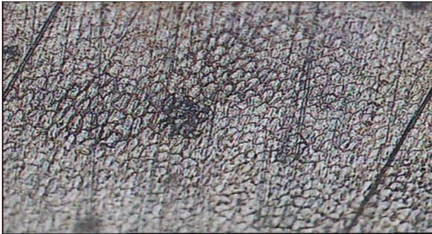
**Figure 2.17** Weldment area (100X magnification : 1.2mm, 30v)
