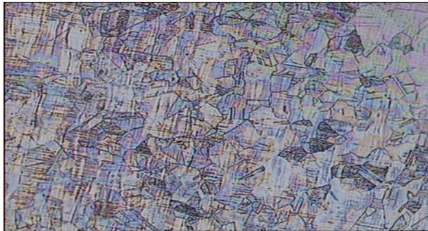
**FIGURE 2.12** HAZ (100X magnification: 0.8mm, 30v)
