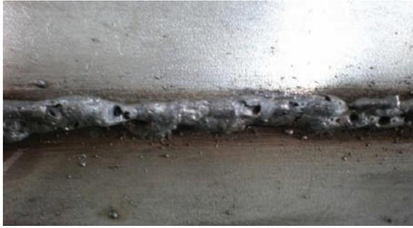
**FIGURE 2.3** Weldment of 1.2mm filler wire diameter
