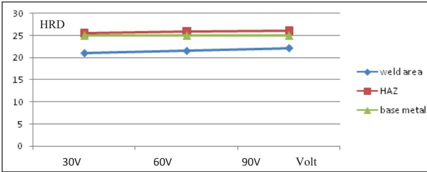
**FIGURE 2.10** Weld area, HAZ and base metal hardness (0.8mm)
