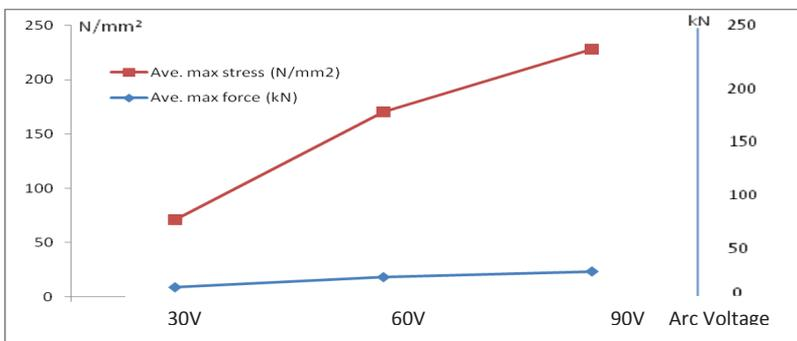
**FIGURE 2.9** Average max force and max stress for 0.8mm filler wire
