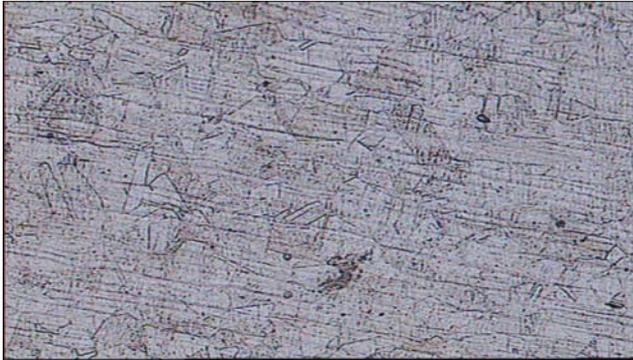
**FIGURE 2.16** HAZ (100X magnification: 1.2mm, 30v)
