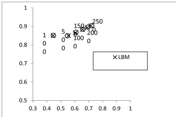
**FIGURE 8** Effect of the Reynolds number to the location of the centre of the primary vortex for isosceles triangular type ‘b’
