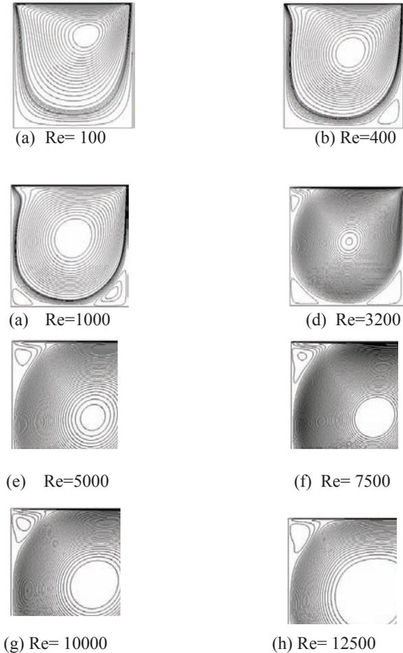
**FIGURE 4** Streamline patterns for lid driven square cavity by using LBM scheme
