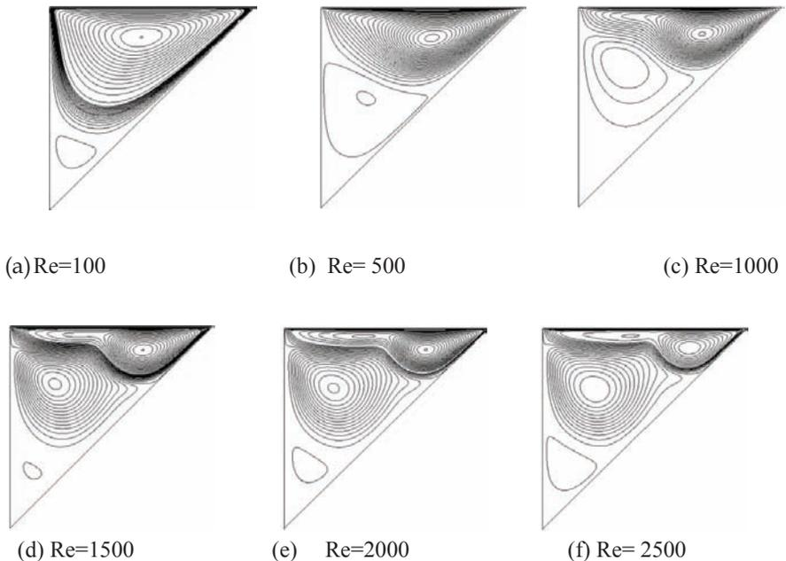
**FIGURE 7** Streamline pattern for isosceles triangular type ‘b’
