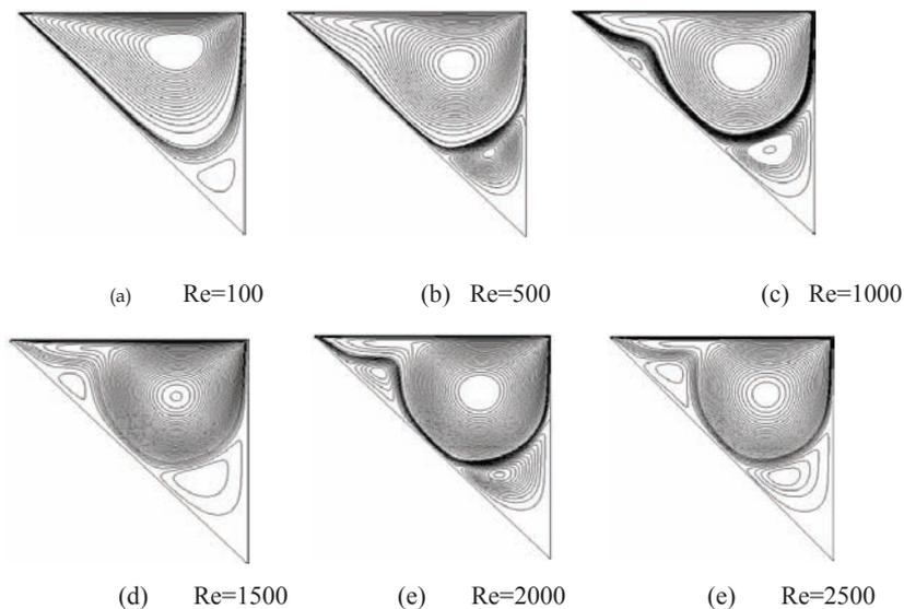
**FIGURE 5** Streamline patterns for isosceles triangular type ‘a’
