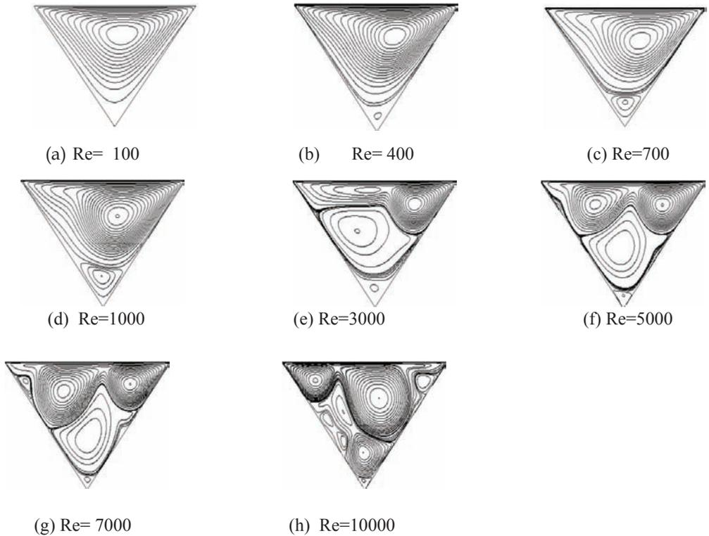
**FIGURE 9** Streamline pattern for isosceles triangular type ‘c’
