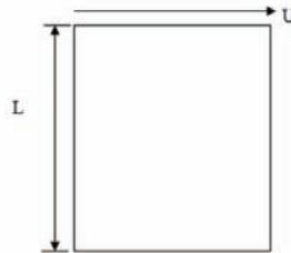
**FIGURE 1** Geometry of shear driven square cavity
