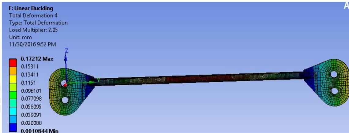
Figure 16(c). Buckling load for SB type 3
