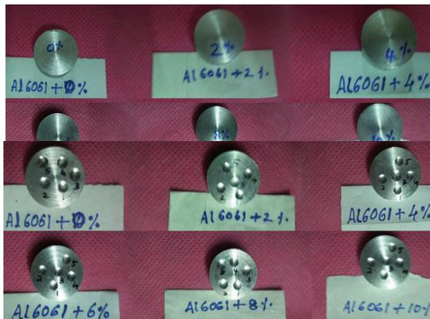
FIGURE 2 Pictorial view of hardness test specimens after indentation
