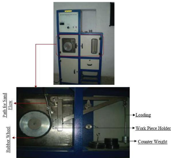
**FIGURE 3** Photograph of sand abrasion testing apparatus
