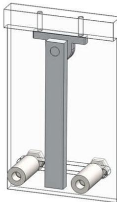
Figure 10. Pendulum-type switch developed for testing its feasibility
