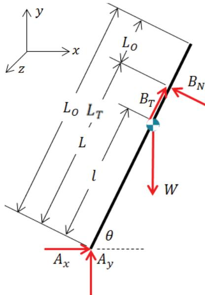
Figure 6. Free body diagram for the ladder in Case II
