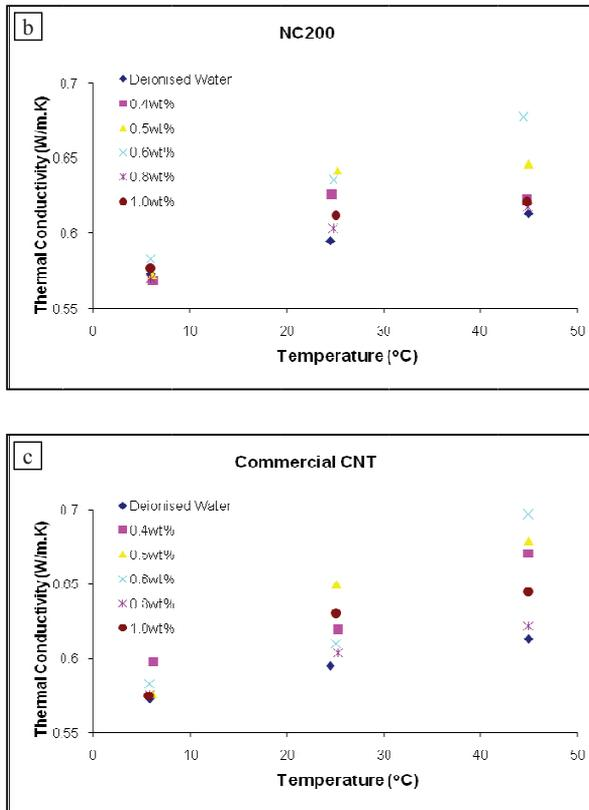
FIGURE 3 Thermal conductivity test for a) NC300, b) NC200, and c) Commercial CNT
