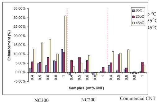
FIGURE 4 Percentage enhancement of nanofluid based nanocarbon
