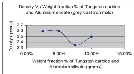
**Figure 4** Density vs Weight fraction % of combined tungsten carbide and aluminium silicate
