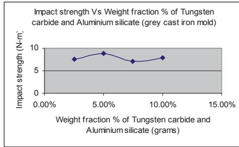
Figure 5 Impact strength vs Weight fraction % of combined tungsten carbide and aluminium silicate
