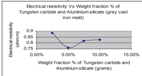
Figure 6 Electrical resistivity vs Weight fraction % of combined tungsten carbide and aluminium silicate
