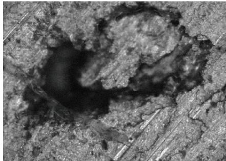
**Figure 9** 5 % Tungsten carbide and aluminium silicate mixed particulate hybrid composite magnified at 50x
