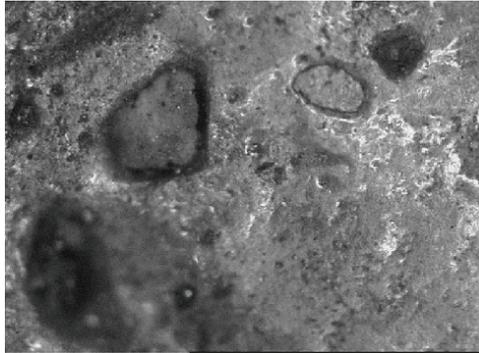
**Figure 8** 2.5 % Tungsten carbide and aluminium silicate mixed particulate hybrid composite magnified at 50x
