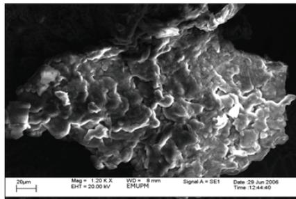
**Figure 15** Interface and bonding in 5% weight fraction of combined tungsten carbide and aluminium silicate particulate reinforced composite magnified at 1200-x
