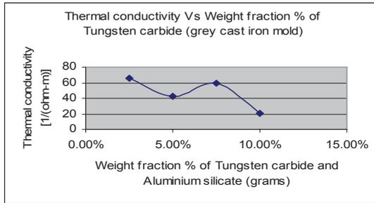
**Figure 7** Thermal conductivity vs Weight fraction percentage of combined tungsten carbide and aluminium silicate
