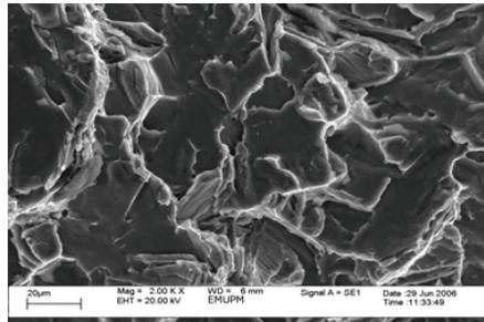
**Figure 13** Tensile fracture surface of 10% weight fraction of combined tungsten carbide and aluminium silicate particulate reinforced hybrid composite magnified at 2000-x
