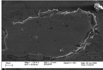
**Figure 14** Interface and bonding in 2.5% weight fraction of combined tungsten carbide and aluminium silicate particulate reinforced composite magnified at 1200-x
