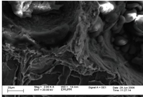
**Figure 11** Tensile fracture surface of 2.5% weight fraction of combined tungsten carbide and aluminium silicate particulate reinforced hybrid composite magnified at 2000 x
