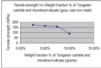
**Figure 1** Tensile strength vs Weight fraction % of combined tungsten carbide and aluminium silicate
