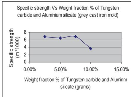
**Figure 2** Specific strength vs Weight fraction percentage of combined tungsten carbide and aluminium silicate
