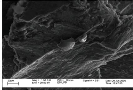
**Figure 16** Interface and bonding in 10% weight fraction of combined tungsten carbide and aluminium silicate particulate reinforced composite magnified at 1500-x
