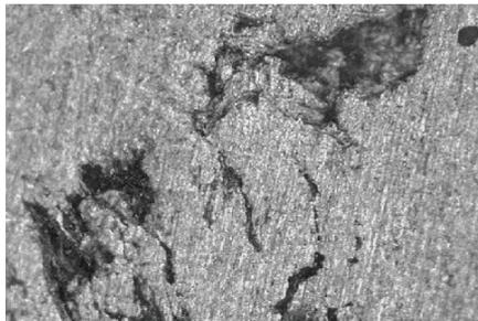
**Figure10** 10 % Tungsten carbide and aluminium silicate mixed particulate hybrid composite magnified at 50 x
