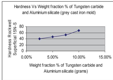
**Figure 3** Hardness vs Weight fraction percentage of combined tungsten carbide and aluminium silicate
