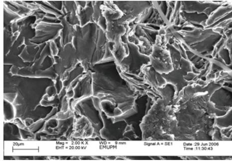
**Figure 12** Tensile fracture surface of 5% weight fraction of combined tungsten carbide and aluminium silicate particulate reinforced hybrid composite magnified at 2000-x
