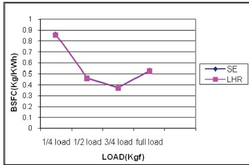
FIGURE 6 Load vs BSFC
