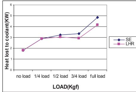
FIGURE 4 Load vs Heat lost to coolant
