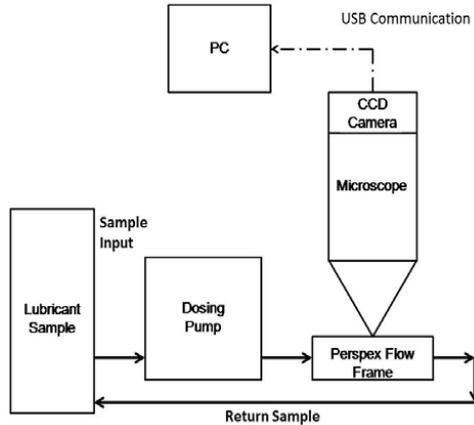
Figure 1. Online working schematic of hardware setup
