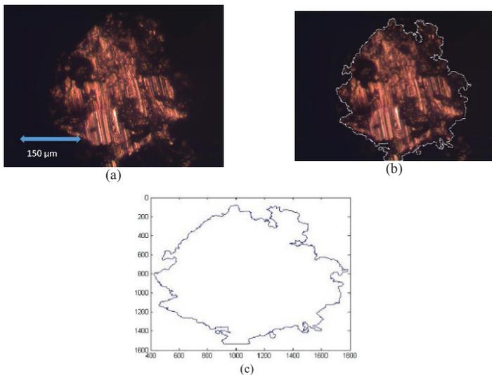
Figure 6. Debris image and processing with lubricant sample 1 (a) Raw debris image, (b) Debris with software sketched boundary and (c) Extracted boundary for RGB values measurement
