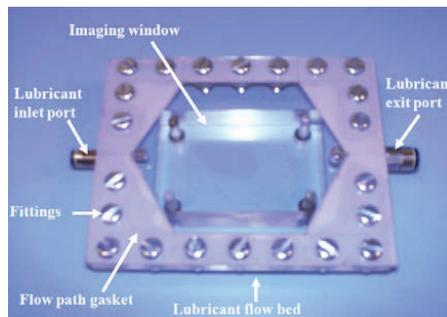
Figure 2. Perspex flow frame
