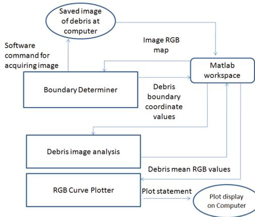
Figure 3. Flow diagram of software with its main components
