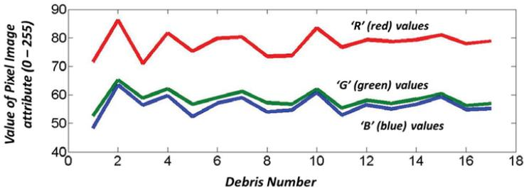
Figure 5. Measured RGB values without the presence of lubricant
