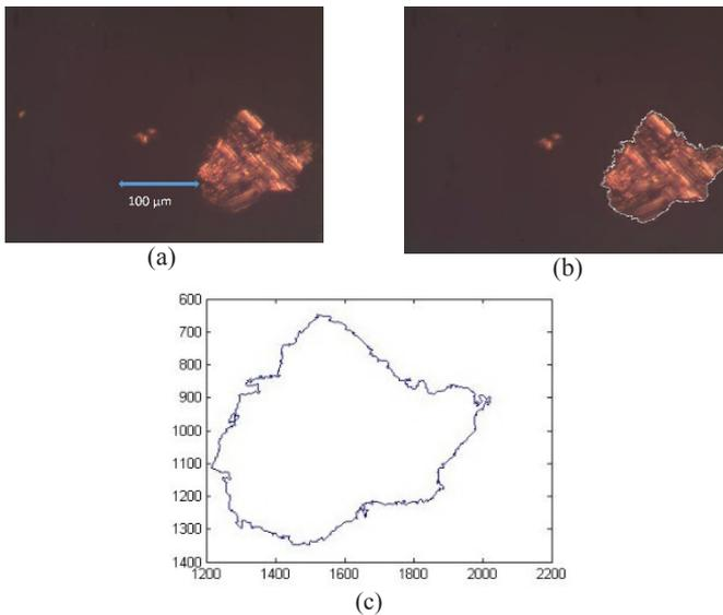
Figure 10. Debris image and processing with lubricant sample 3 (a) Raw debris image, (b) Debris with software sketched boundary and (c) Extracted boundary for RGB values measurement
