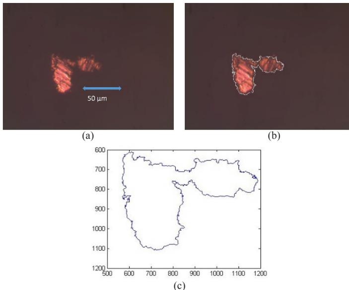
Figure 8. Debris image and processing with lubricant sample 2 (a) Raw debris image, (b) Debris with software sketched boundary and (c) Extracted boundary for RGB values measurement
