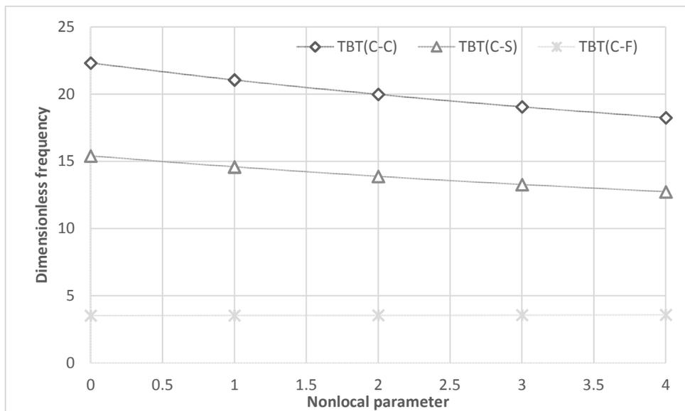
Figure 5. Non-dimensional fundamental frequencies of different edge conditions ( $L/h = 50$ )
