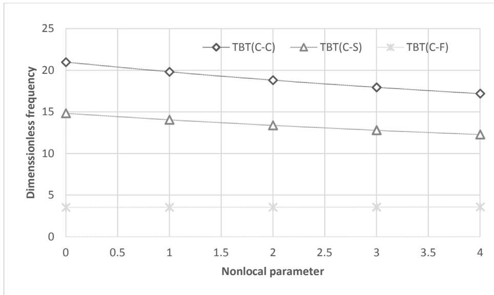
Figure 4. Non-dimensional fundamental frequencies of different edge conditions ( $L/h = 10$ )
