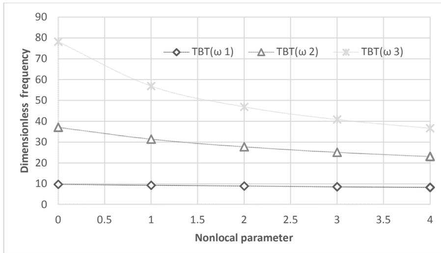
Figure 2. Non-dimensional natural frequencies of S-S nanobeams ( $L/h = 10$ )
