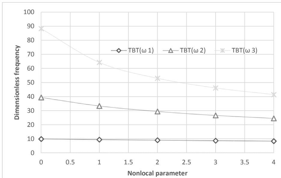
Figure 3. Non-dimensional fundamental frequencies of S-S nanobeams ( $L/h = 50$ )
