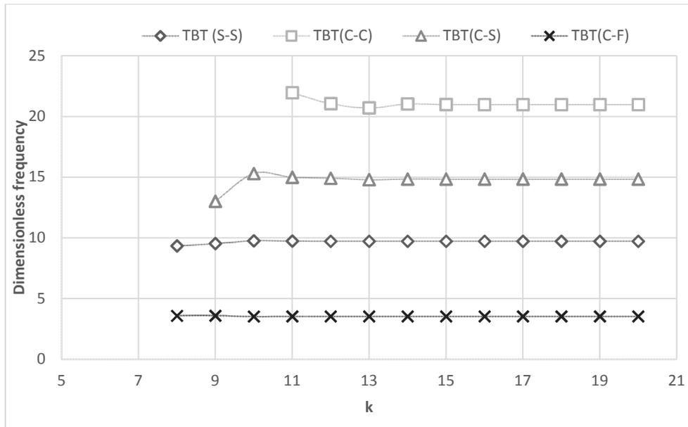
Figure 1. Convergence study of fundamental frequencies of Timoshenko nanobeam with various edge conditions ( $L/h = 10$ ,  $\mu = 0$ )
