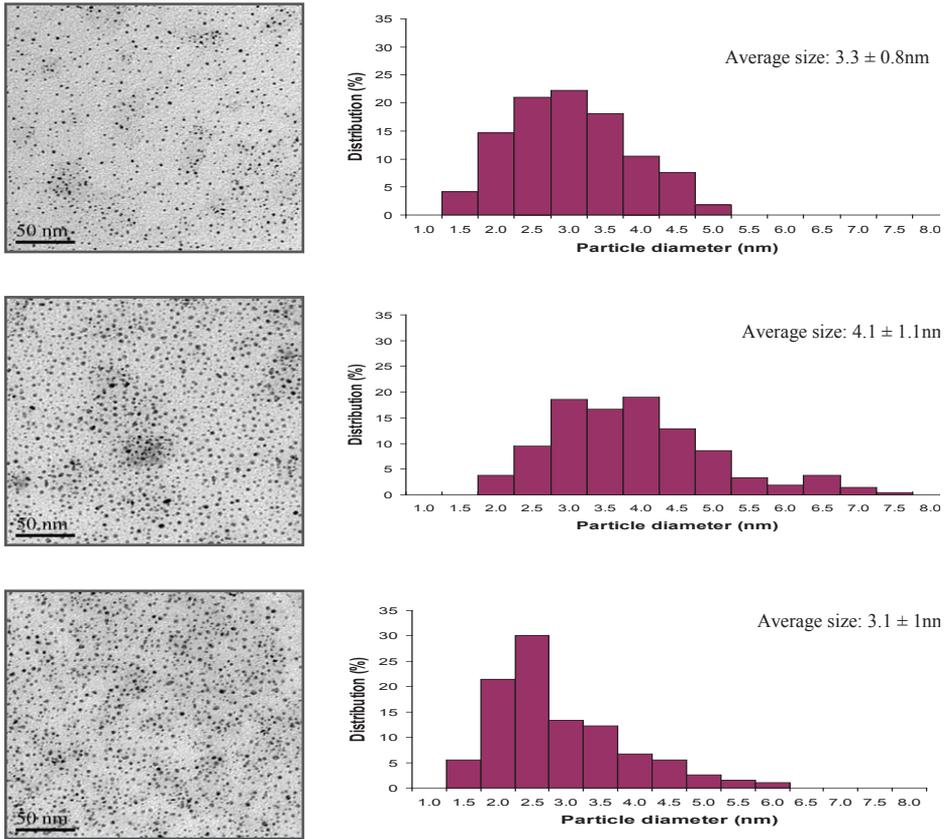
Figure 2. The TEM image and particle size distribution of (a) Pt-Cu (1:1)-mw, (b) Pt-Cu (1:1)-NaBH<sub>4</sub> and (c) Pt-Cu (1:1)-comb
