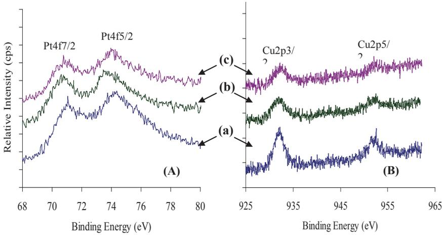
Figure 4. XPS peaks of Pt 4f (A) and Cu 2p (B) for (a) Pt-Cu (1:1)-mw, (b) Pt-Cu (1:1)-NaBH<sub>4</sub> and (c) Pt-Cu (1:1)-comb
