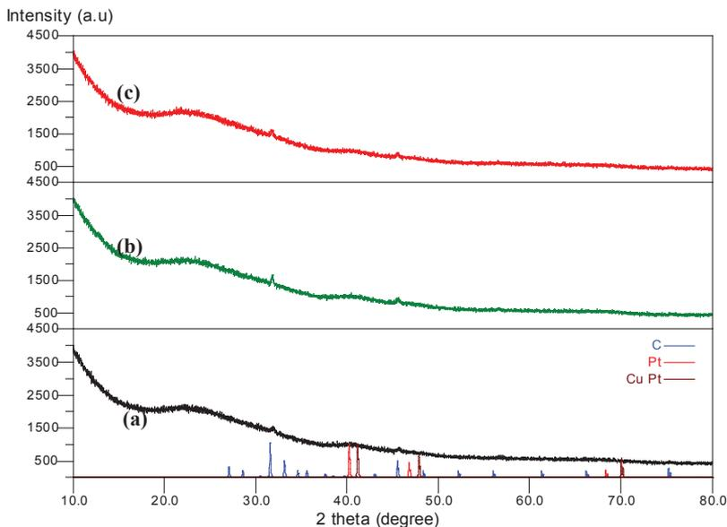
Figure 3. The XRD pattern of (a) Pt-Cu (1:1)-mw, (b) Pt-Cu (1:1)-NaBH<sub>4</sub> and (c) Pt-Cu (1:1)-comb
