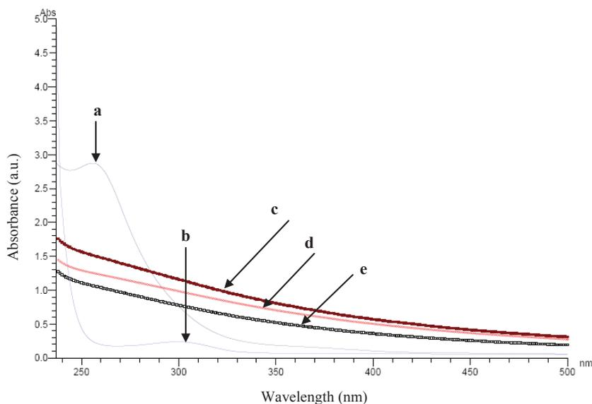
Figure 1. UV-vis absorption spectra of (a) Pt ion, (b) Cu ion, (c) Pt-Cu (1:1)-mw, (d) Pt-Cu (1:1)-NaBH<sub>4</sub> and (e) Pt-Cu (1:1)-comb
