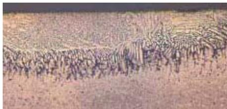
Figure 1 Optical micrograph of the NiTi-NiTi plasma weld [25]
