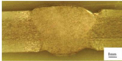
Figure 7 Experimental cross-section in keyhole double-sided arc welding [78]
