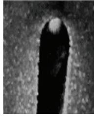
Figure 6 Simultaneous imaging of weld pool and keyhole [72]
