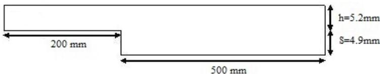
Figure 6. Geometric model of back ward facing step
