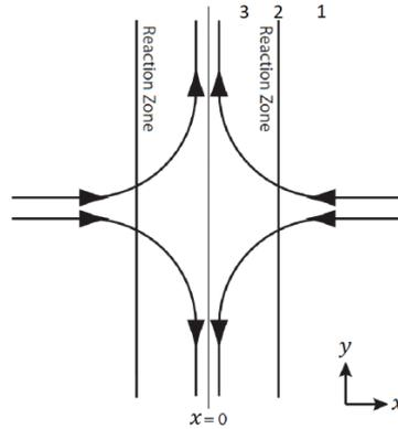
Figure 1 The counterflow configuration and twin planar premixed flames
